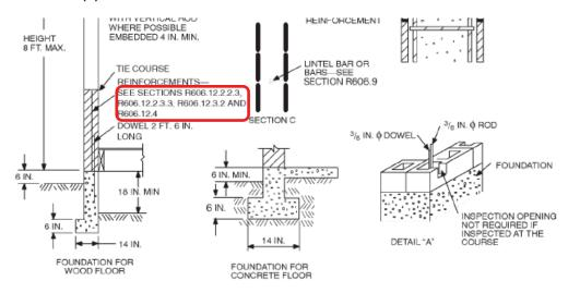
NOTE: A full bed joint must be provided. All cells containing vertical bars are to be filled to the top of wall and provide inspection opening as shown on detail "A."
