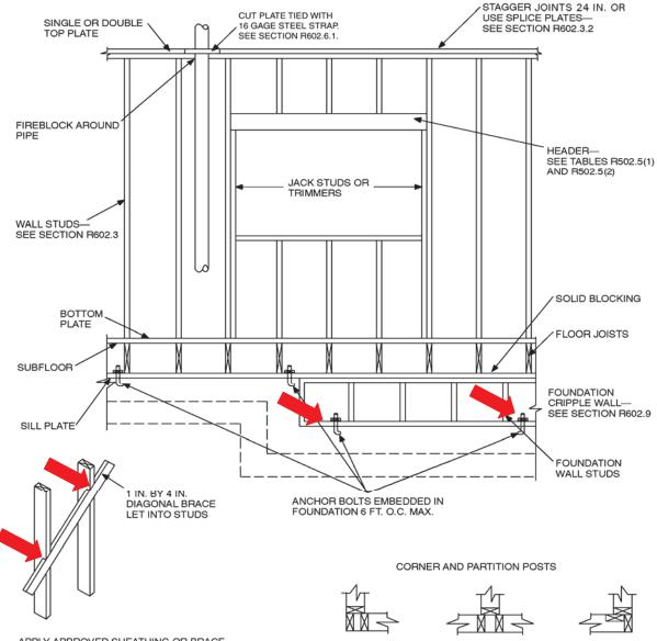
APPLY APPROVED SHEATHING OR BRACE EXTERIOR WALLS WITH 1 IN. BY 4 IN. BRACES LET INTO STUDS AND PLATES AND EXTENDING FROM BOTTOM PLATE TO TOP PLATE, OR OTHER APPROVED METAL STRAP DEVICES INSTALLED IN ACCORDANCE WITH THE MANUFACTURER'S SPECIFICATIONS, SEE SECTION R602.10.
