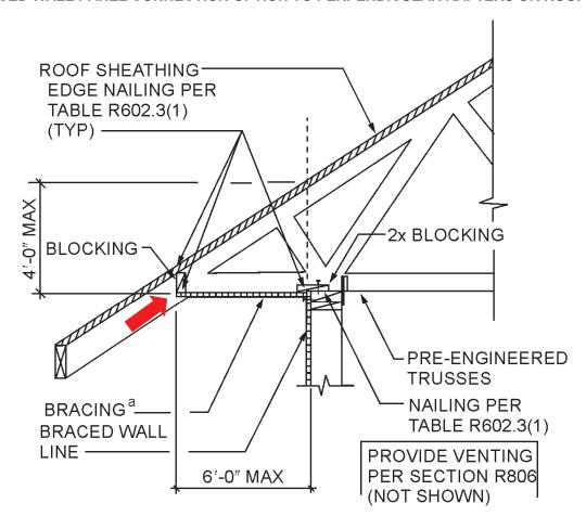
a. METHODS OF BRACING SHALL BE AS DESCRIBED IN SECTION R602.10.2 METHOD DWB, WSP, SFT, BG, PBS, PCP OR HPS
