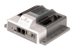
Cortex microcontroller, ARM cpu with multiple I/O ports, stores and runs programs
