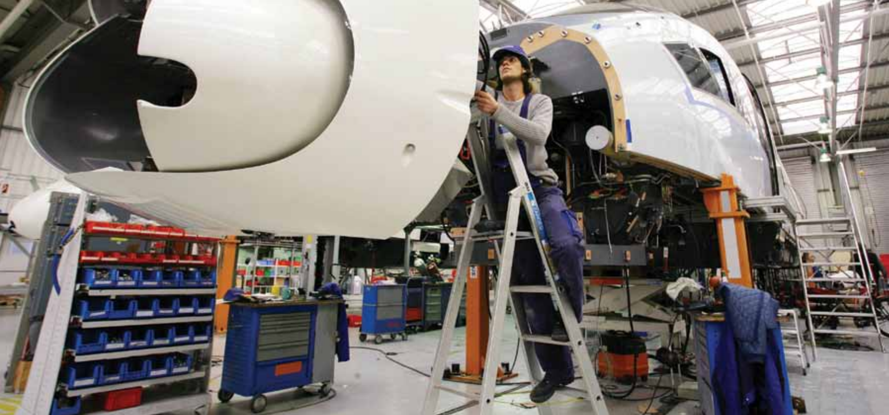
Workers building a high-speed train at a Siemens plant in Krefeld, Germany.
