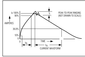
Figure 5. Human Body Model Current Waveform
