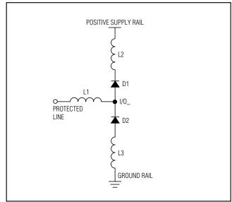
Figure 1. Parasitic Series Inductance
