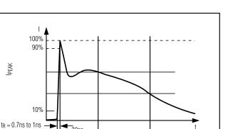
Figure 3. IEC 61000-4-2 ESD Generator Current Waveform
