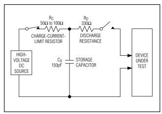
Figure 6. IEC 61000-4-2 ESD Test Model
