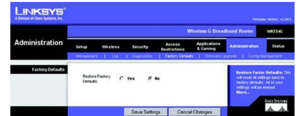
Figur 5-43: Fanen Administration - Factory Defaults (Administration - Fabriksindstillinger)
