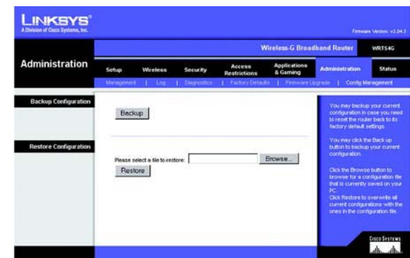
Figur 5-45: Fliken Administration – Config Management (Konfigurationshantering)
