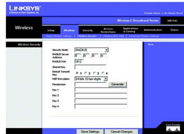
Figure 5-22: Wireless Tab - Wireless Security (RADIUS)
