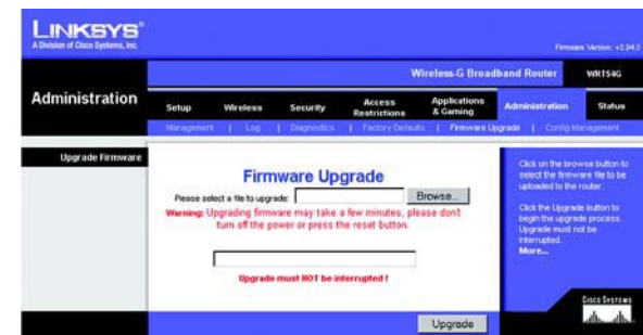
Figuur 5-44: Tabblad Administration (Administratie) - Firmware Upgrade (Firmware-upgrade)
