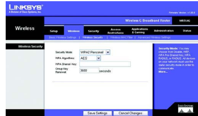
Figure 5-20: Wireless Tab - Wireless Security (WPA2 Personal)
