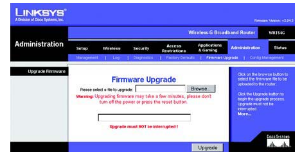
Figur 5-44: Fliken Administration – Firmware Upgrade (Uppgradera fast programvara)
