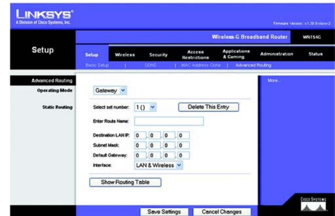
Figur 5-15: Fliken Setup (Konfiguration) – Advanced Routing (Avancerad routing) (Gateway)
