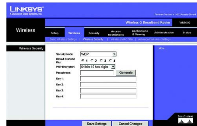
Abbildung 5-23: Registerkarte „Wireless“ – „Wireless Security (WEP)“ (Wireless-Sicherheit (WEP))
