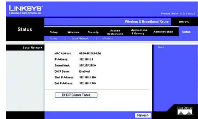
Figure 5-47: Status Tab - Local Network
