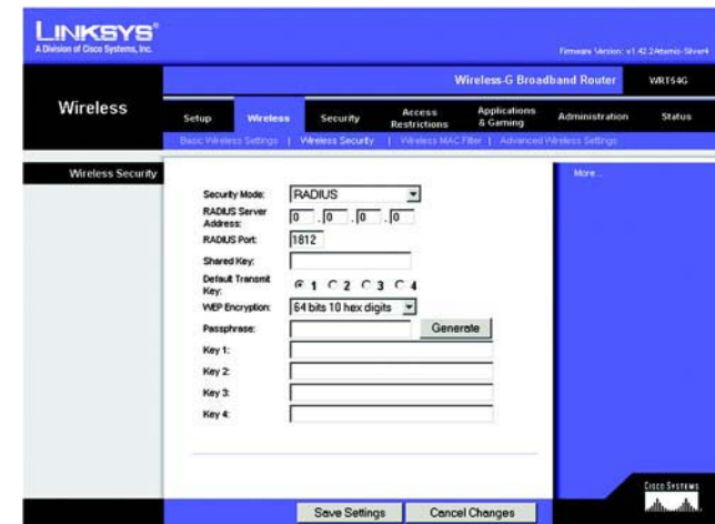
Figure 5-22 : Onglet Wireless - Wireless Security (RADIUS) (Sans fil - Sécurité sans fil [RADIUS])
