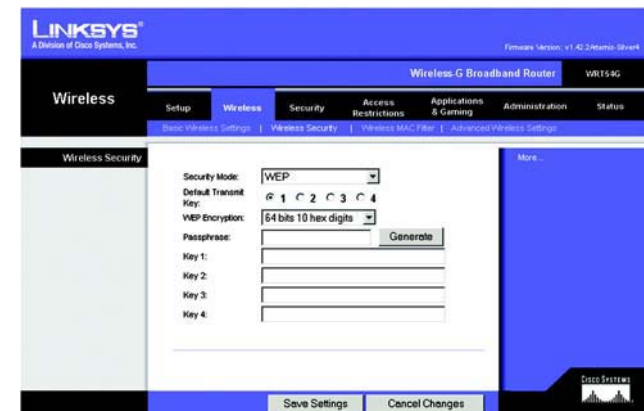
Figure 5-23: Wireless Tab - Wireless Security (WEP)
