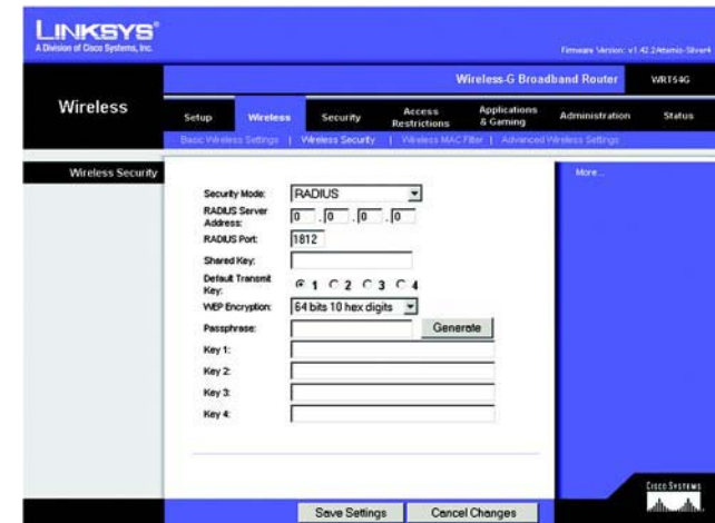
Abbildung 5-22: Registerkarte „Wireless“ – „Wireless Security (RADIUS)“ (Wireless-Sicherheit [RADIUS])
