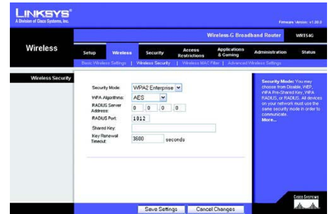
Figuur 5-21: Tabblad Wireless (Draadloos) - Wireless Security (WLAN-beveiliging) (WPA2 Enterprise)
