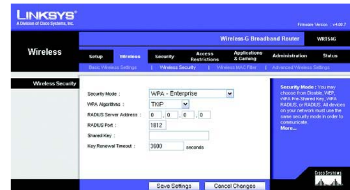
Figure 5-19: Wireless Tab - Wireless Security (WPA Enterprise)
