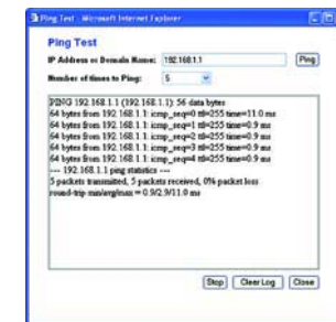
Figure 5-41 : Ping Test (Test Ping)
