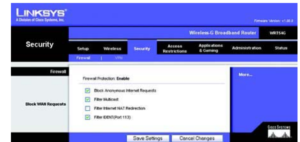
Figur 5-27: Fanen Security - Firewall (Sikkerhed - Firewall)
