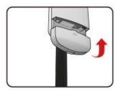
Align the base with the weatherproof sliding door.
