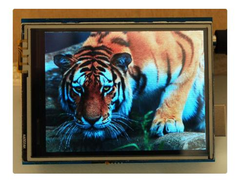
To make new bitmaps, make sure they are less than 240 by 320 pixels and save them in 24-bit BMP format! They must be in 24-bit format, even if they are not 24-bit color as that is the easiest format for the Arduino. You can rotate images using the setRotati on() procedure.
