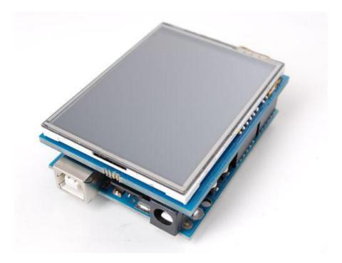
Because the TFT is exactly the same size as an Arduino, we preassemble the shield in the factory. To use, simply place it onto your Arduino. No wiring, no soldering!
