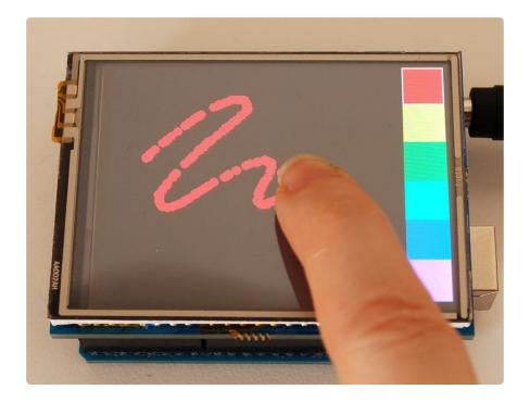
Spice up your Arduino project with a beautiful large touchscreen display shield with built in microSD card connection. This TFT display is big (2.8" diagonal) bright (4 white-LED backlight) and colorful (18-bit 262,000 different shades)! 240x320 pixels with individual pixel control. It has way more resolution than a black and white 128x64 display. As a bonus, this display has a resistive touchscreen attached to it already, so you can detect finger presses anywhere on the screen.
