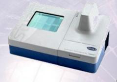
Melting point apparatus
