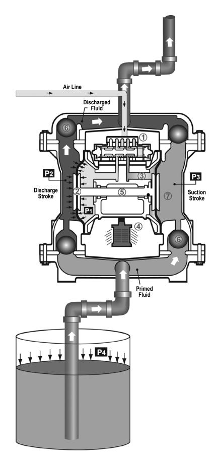
VERSA-MATIC<sup>®</sup> e2mdlCsmATEXAB-rev0514 Air-Operated Double Diaphragm (AODD) pumps are powered by compressed air or nitrogen.
