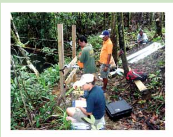
EQPB Staff undertaking cableway gauging on the Tabecheding River
