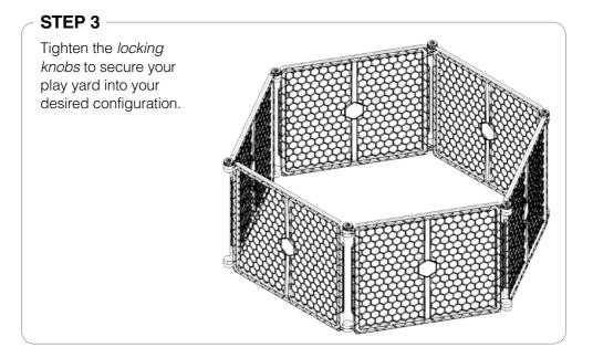
**NOTE:** When adding or removing additional panel units to the configuration, panels must be added or subtracted in sets of two for the freestanding enclosure to function properly.
