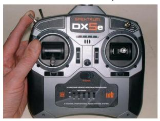
**2.2** Set the DX5e **Mode # 2** channel # 5 switch on the TX to # 1 ON, i.e. pull switch towards you.
