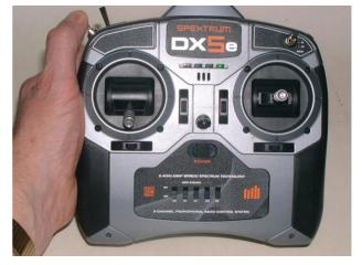
**2.6** Turn the Channel # 5 switch to "0" OFF. i.e. push switch away from you.
