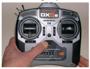
**2.3** Turn the TX ON. RH LED will illuminate. Make sure Throttle stick is down. Zero output.
