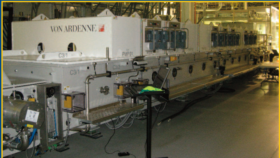
(2) VON ARDENNE SPUTTERING LINE W/ CARDINAL LOADING SYSTEMS, (LONGMONT LOCATION)
