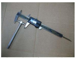
Figure 2.4.3: Telescoping Gauge and Vernier Caliper
