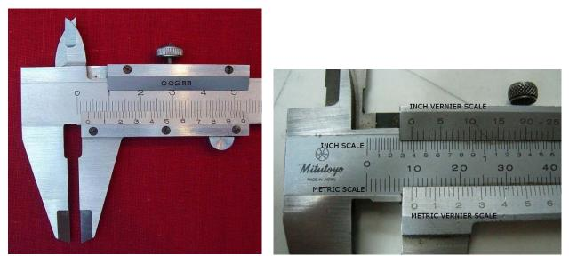
Figure 2.3.2: Metric Vernier Caliper
