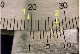
Figure 2.3.6: Angular Vernier Scale
