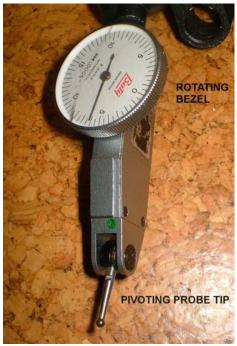
Figure 2.4.6: Dial Test Indicator
