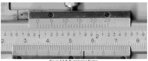
Figure 2.3.7: Dual Vernier Scales
