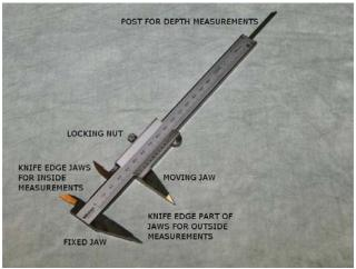
Figure 2.3.4: Components of a Vernier Caliper
