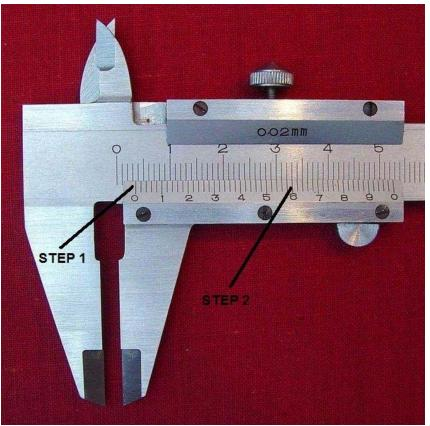
Figure 2.3.5: Reading Vernier Scales
