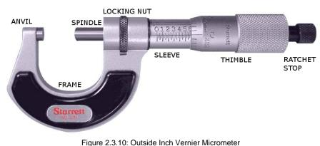
The spindle should only be moved using the ratchet stop and not the thimble to prevent any damage to the hardened spindle and anvil faces due to excessive pressure. The ratchet stop contains a slip clutch which will begin to slip at the proper pressure, thus also
