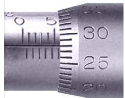
Figure 2.3.14: Metric Micrometer Scales
