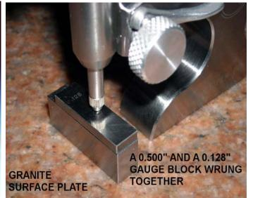
Figure 24.8: Wrung Gauge Blocks
