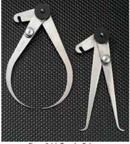
Figure 2.4.1: Transfer Calipers
