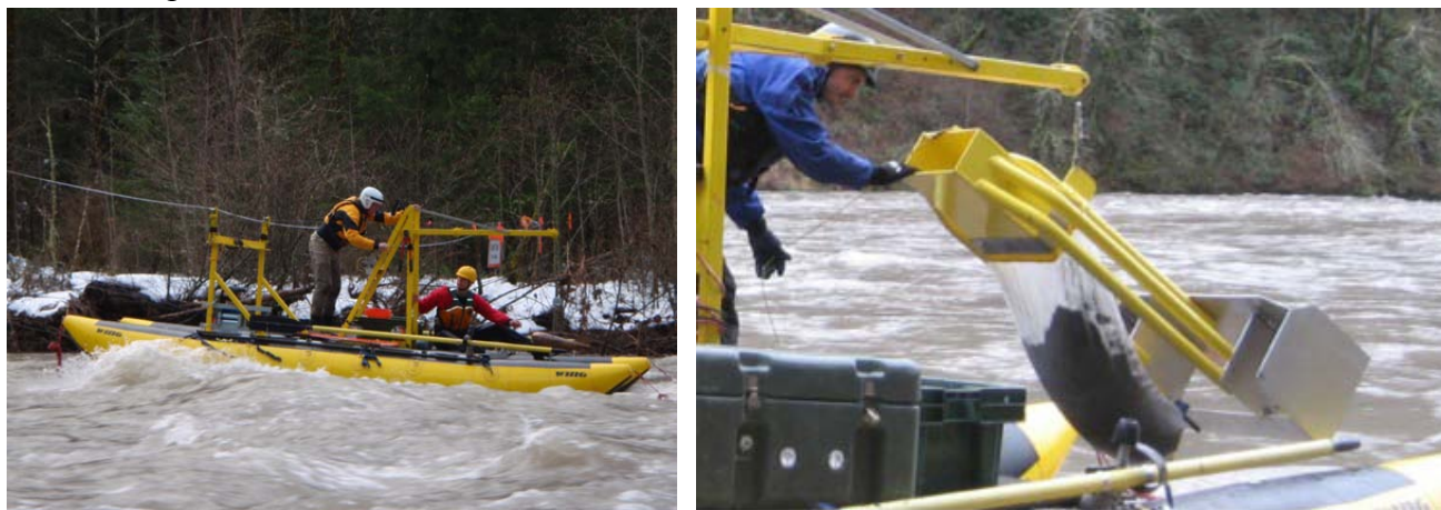
Figure 29 – Sediment sampling from the cataraft on a cableway platform (left) with the TR2 Bedload Sampler (right).
