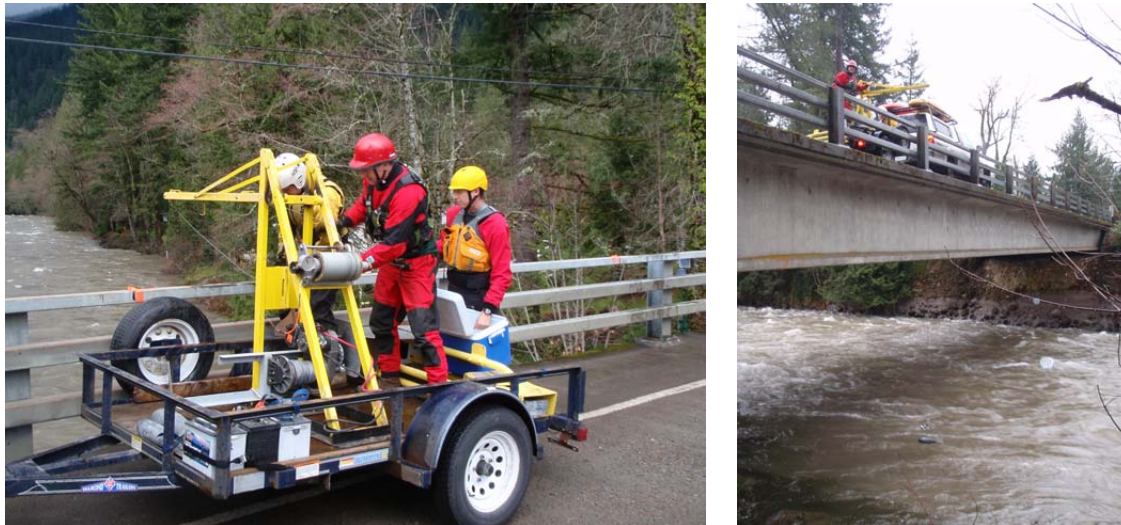
Figure 30 – Bridge crane sampling setup.
