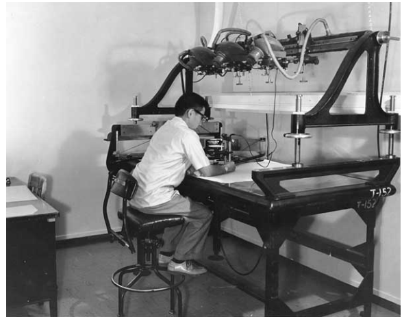
Figure 43. ER-55 Plotter developed by Bean at the USGS.
