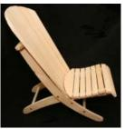
The chair is now assembled, and ready for finishing. If you are painting the chair, it is best to prime all surfaces first before assembly, to ensure longer life against moisture. Use an oil based paint like Varathane Colors, for the final coat. You can either countersink and plug the screw holes before final painting, or use brass screws left exposed if staining.
