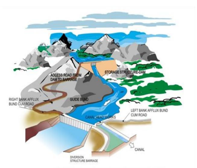
FIGURE 1. Structures for harnessing water resources potential of a river
