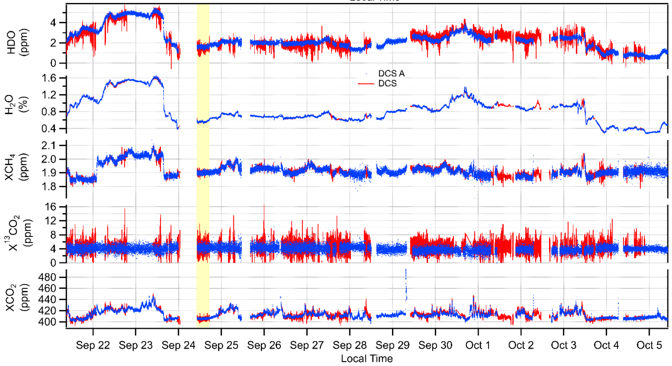
Figure 5. Concentration retrievals from DCS A (blue dots) and DCS B (red lines) for HDO (% by volume)(ppm) H 2 O (% by volume),(%), dry CH 4 , dry CO 2 and dry 13 CO 2 over two weeks at 30-second intervals. Excellent agreement is observed between both systems for all species, though it is clear that over this path length 13 CO 2 does not provide a strong enough signal to retrieve reliably. Highlighted section: 6-hour, well-mixed period over which Allan deviations (Figure 8) are calculated. Missing data is primarily due to telescope misalignment and less frequently, phase lock by one of the combs.
