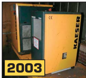
2003 Kaeser TB-19 Compressor & Air Dryer
