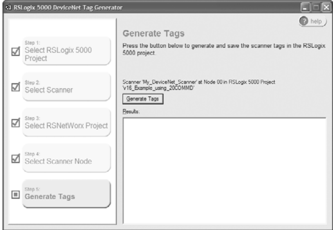
Figure 4.20 RSLogix 5000 DeviceNet Tag Generator Step 5 Window
