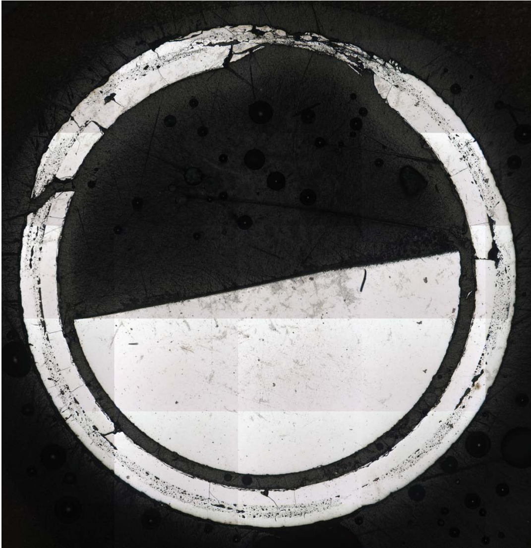
Figure 14. Cross section of top end plug and adjacent cladding. Note the poor condition of the cladding and the uneven distribution of the fibers at the 5 o'clock position. The end plug either shifted or chipped and could not be polished flat. The cement holding the plug in is not readily apparent. The black regions are epoxy; it is difficult to tell if the SiC composite has significant porosity or if these regions are due to pull-out during preparation.
