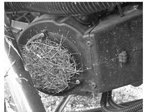
Debris clogging the cooling fan
