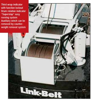
The ATC-3200's powerful, responsive and productive winches generate the strongest winch line pull in its class with 21,010 lbs (9 530.0 kg) and a winch line speed of 526 fpm (160.21 m/min). Piston motors provide precise movement at any speed.
