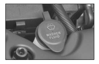
The windshield washer fluid reservoir is located in front of the fuse block relay center on the passenger's side of the vehicle.
