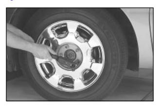
Using the wheel wrench, loosen all the wheel nuts. Don't remove them yet.
