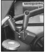
8. Don't let the other end of the positive (+) cable touch metal. Now, connect the red + terminal to the red positive (+) terminal of the other vehicle's battery. Use a remote positive (+) terminal if the vehicle has one.
