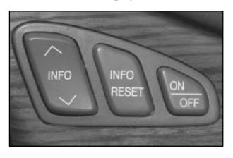
INFO: Pressing this button up or down will display the MILES RANGE (Analog Cluster), MPG AVG, MPG INST, GAL FUEL USED, AVG MPH, TIMER, BATTERY VOLTS, RPM TACHOMETER (Digital Cluster), ENGINE OIL LIFE, TRANS FLUID LIFE, PHONE (If Equipped), FEATURE PROGRAMMING and Blank Display.
