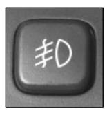
Use the fog lamps for better vision in foggy or misty conditions. When you press the fog lamp button, a fog lamp symbol located in the instrument panel will come on to indicate that the fog lamps and the parking lamps are on.
