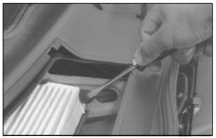
2. Then, insert the flat tip of the screwdriver behind the push pin located on the inboard side of the air filter compartment to carefully pry the pin out.
