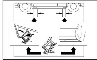
2. Find the jacking location from the diagrams above and corresponding hoisting notches located in the plastic molding. The notches may be labeled "JACK" with an arrow pointing to the jacking location on the vehicle.
