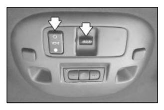
The two control switches to operate the sunroof are located on the overhead console and include VENT, open and close.
