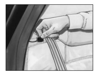
1. Remove the guide from its storage pocket on the top of the seatback.
