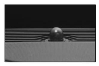
The sensor monitors the sun's solar radiation and is located on top of the instrument panel near the windshield. The ECC panel uses this information to automatically make the necessary temperature and airflow adjustments to maintain your comfort.
