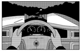
Remember that the Night Vision System can only help you see objects that are warmer or colder than the surroundings. It can't sense things like brake lights, turn signals or emergency flashers, traffic lights or signs.
