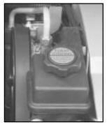
The power steering fluid reservoir is located between the fuse block relay center and the engine on the passenger's side of the vehicle.
