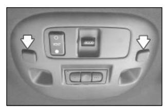
These lamps are located in the front overhead console. Press the button to turn them on. Press it again to turn them off.
