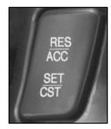
The controls to operate cruise control are located on the steering wheel.
