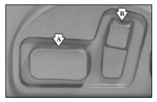
Press the recliner control (B), located on the side of the seat, forward or rearward to adjust the seatback.
