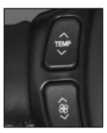
Some heating and cooling controls can be adjusted at the steering wheel. Other touch controls operate some audio controls. See "Audio Steering Wheel Controls" in the Index.
