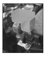
5. Lift and move the red positive (+) terminal cover away from the relay center.
