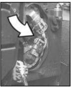
6. Turn the headlamp housing socket counterclockwise to unlock the socket from the lamp housing.
