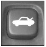
To use this feature, your vehicle must be in PARK (P) or NEUTRAL (N) and the VALET lockout switch must be off.
