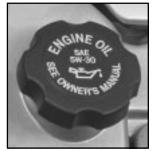
The oil fill cap is located behind the radiator on the passenger's side of the engine. Turn the cap counterclockwise to remove it.
