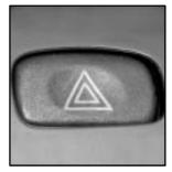
The hazard warning button is located on the center of the instrument panel between the two air yents.
