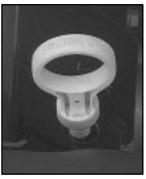
The engine oil dipstick is located behind the radiator on the driver's side of the engine. The handle says ENGINE OIL on it.
