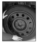
9. Place the spare tire on the wheel-mounting surface.
