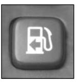
The fuel door release button is located to the left of the steering wheel next to the headlamp knob.
