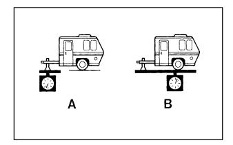
If you're using a weight-carrying hitch, the trailer tongue (A) should weigh 10 percent of the total loaded trailer weight (B). If you have a weight-distributing hitch, the trailer tongue (A) should weigh 12 percent of the total loaded trailer weight (B).
