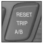
Press this button, to tell how far you've traveled since you last set the trip odometer back to zero.
