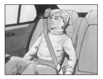
Buckle, position and release the safety belt as described in "Rear Seat Passenger Positions" earlier in this section. Make sure that the shoulder belt crosses the shoulder.
