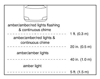
A chime will sound the first time an object is detected. URPA can detect objects 3 inches (7.6 cm) and wider, and at least 10 inches (25.4 cm) tall, but it cannot detect objects that are above trunk level. In order for the rear sensors to recognize an object, it must be within operating range.
