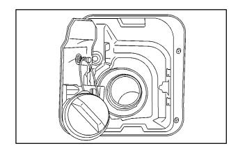
While refueling, hang the cap by the tether from the hook on the filler door.
