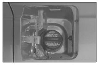
The cap is located behind a hinged door on the driver's side of your vehicle.
