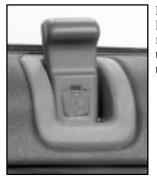
Push down on the manual lock button to lock the door from the inside. To unlock the door, pull up on the button.
