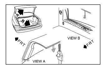
This feature is used to secure the trunk lid if it will not close completely, such as when carrying large packages in the trunk.
