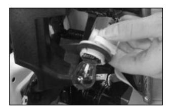
3. Remove the turn signal lamp housing socket and replace the bulb.
