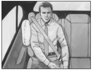
The side impact air bags for the rear seat outboard passenger positions are in the sides of the rear seatback closest to the doors.
