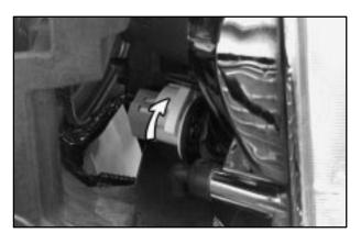
Press the tab down and turn the housing socket clockwise to unlock the socket from the lamp housing.
