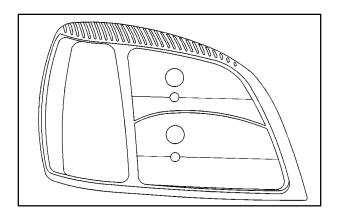
Measure the distance from the ground to the aim dot on each lamp; if left low beam, subtract two inches. Record this distance. 3. At the wall or other flat surface, measure from the floor to the recorded distance and draw a horizontal line the width of the vehicle.
