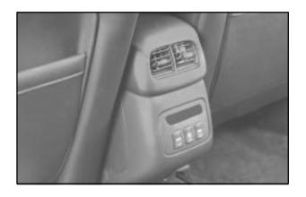
Your vehicle is equipped with a rear climate control. With this system, the rear passengers can control the
