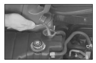
The surge tank is located on the passenger's side of the engine.
