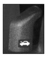
Pull the lever inside the vehicle to open the hood. It is located on the lower driver's side of the instrument panel.
