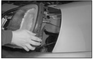
4. Firmly grasp the outboard side of the headlamp assembly with both hands and pull hard enough, so that the whole assembly opens freely.
