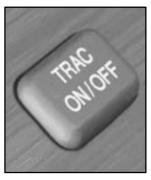
To turn the system off, press the button located on the center console. (For vehicles with a column shifter, the button is located at the end of the shift lever.) The TRACTION OFF message will display on the Driver Information Center. If the system is limiting wheel spin when you press the button, the TRACTION OFF message will display -- but the system won't turn off right away. It will wait until there's no longer a current need to limit wheel spin.
