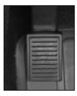
Hold the regular brake pedal down with your right foot and push the parking brake pedal down with your left foot to set the parking brake.
