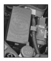
The front Bussed Electrical Center (BEC) is located next to the engine on the passenger's side of the vehicle.
