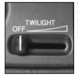
This control is next to the headlamp knob. It automatically switches the lamps on and off by sensing how dark it is outside.
