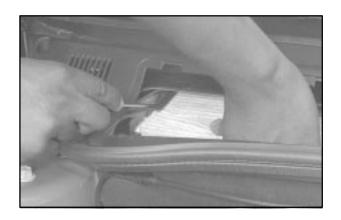
3. To remove the air filter, insert the flat tip of the screwdriver between the air filter and the compartment wall on the outboard side of the vehicle. Then, push in to flatten the pin holding the air filter in place. Gently remove the air filter and any loose debris that may be inside the air filter compartment.
