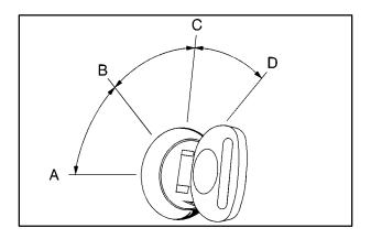
With the ignition switch, you can turn the switch to four different positions.
