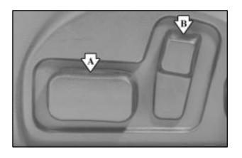
The power seat controls, located on the sides of the front seats, move and adjust the angle of the front seats.
