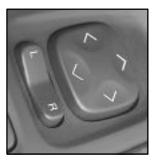
The control on the driver's door armrest operates both outside rearview mirrors. Press (R) on the control switch to choose the right mirror or (L) to choose the left mirror. The center switch position is for off and will not move the mirrors if touched.
