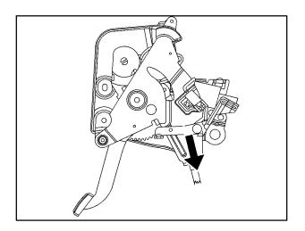
Reach under the driver's side of the instrument panel and pull on the manual release lever, which is located above the parking brake pedal. If the parking brake does not release, you should either drive to the nearest service station or have your vehicle towed.
