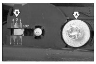
Once the horizontal aim is adjusted, then adjust the vertical aim.
