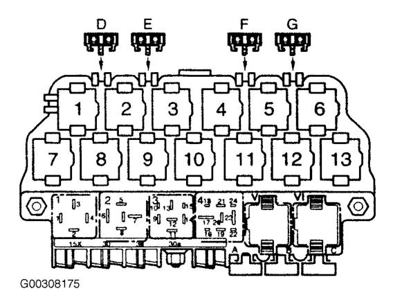
Fig. 9: Identifying Thirteenfold Auxiliary Relay Panel Courtesy of VOLKSWAGEN UNITED STATES, INC.
