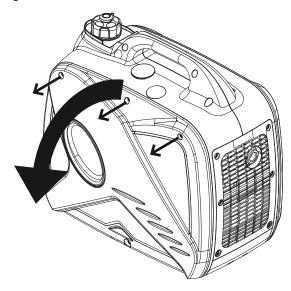
2. Remove the screw, and then the Air Filter Cover and air filter elements. Check for dirt. Clean as described below.
