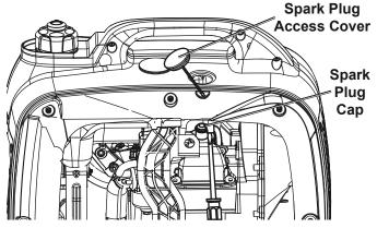
Remove Spark Plug Access Cover from top of Generator. 4. Using a spark plug wrench through the port in the top of the Generator, remove the spark plug.
