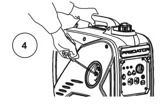
Allow the Engine to run for several seconds.
