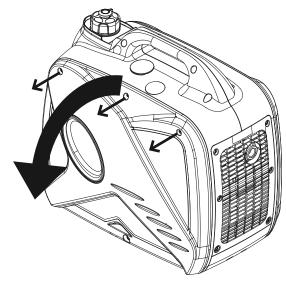
Disconnect spark plug cap from end of plug. Clean out debris from around spark plug.
