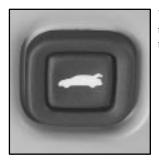
You can also unlock the trunk from inside the vehicle.
