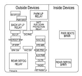
**Circuit Relay** PARK LP RELAY BACKUP LP RELAY BATT RUN DOWN PROTECTION RELAY REAR DEFOG RELAY
