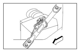
In very cold weather,  $0^{\circ}F(-18^{\circ}C)$  or colder, the engine coolant heater can help. You'll get easier starting and better fuel economy during engine warm-up. Usually, the coolant heater should be plugged in a minimum of four hours prior to starting your vehicle.
