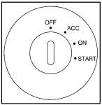
The ignition switch is located on the instrument panel, to the right of the steering column.
