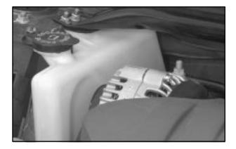
The coolant recovery tank is located between the power steering fluid reservoir and the underhood fuse block on the passenger's side of the engine compartment. See "Engine Compartment Overview" in the Index for more information on location. The vehicle must be on a level surface. When your engine is cold, the coolant level should be at the COLD mark or a little higher. When your engine is warm, the level should be up to the HOT mark or a little higher.
