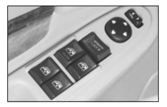
Switches located on the driver's door armrest control each of the windows when the ignition is in ON, ACC, or when retained accessory power (RAP) is active. In addition, each passenger's door has a window switch.
