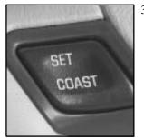
3. Press the SET button on your steering wheel and release it.
