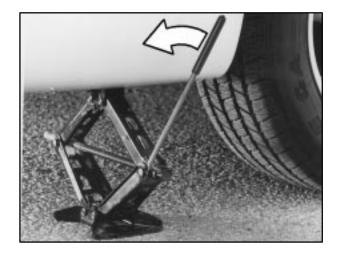
6. Lower the vehicle by turning the jack handle counterclockwise. Lower the jack completely.
