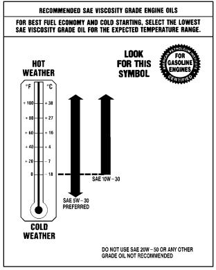
As in the chart shown previously, if you have the 3400 V6 engine, SAE 5W-30 is best for your vehicle. However, you can use SAE 10W-30 if it's going to be  $0^{\circ}$ F (-18°C) or above. These numbers on an oil container show its viscosity, or thickness. Do not use other viscosity oils, such as SAE 20W-50.
