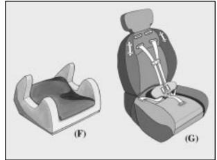
A forward-facing child seat (C-E) provides restraint for the child's body with the harness and also sometimes with surfaces such as T-shaped or shelf-like shields. A booster seat (F-G) is a child restraint designed to improve the fit of the vehicle's safety belt system. Some booster seats have a shoulder belt positioner, and some high-back booster seats have a five-point harness. A booster seat can also help a child to see out the window.
