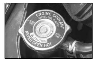
The radiator pressure cap is located in the front of the engine compartment on the passenger's side, near the diagonal cross brace. See "Engine Compartment Overview" in the Index for more information on location.
