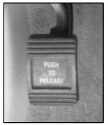
The parking brake is located to the left of the brake pedal, near the driver's door.
