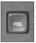
To turn the fog lamps on, press the fog lamps button located next to the exterior lamp control on the left side of the steering column. Your ignition must be in ON for the fog lamps to illuminate.
