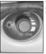
The lamp controls are located on the instrument panel.
