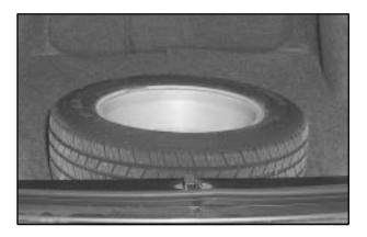
When storing a full-size tire, you must use the extension to help avoid wheel surface damage. Use the extension and protector/guide located in the foam holder. To store a full-size tire, place the tire in the trunk valve stem facing down with the protector/guide through a wheel bolt hole. Remove the the protector and attach the retainer securely. Please note that the cover will not fit over a full-size tire, so be sure to store the cover as far forward as possible.
