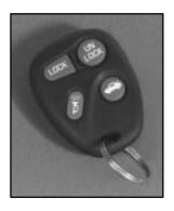
Press UNLOCK once to unlock the driver's door and to turn on the interior lamps. (See "Illumination on Remote Activation" in the Index for more details).
