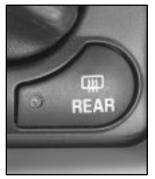
Press the button marked REAR to turn the defogger on. An indicator on the button will light.
