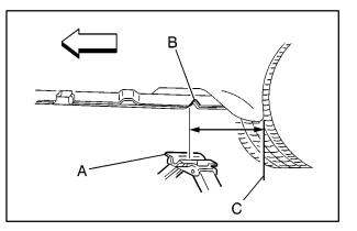
The diagram shows you where you should place your jack. Use the bolts (A) as a guide when positioning the jack lift head (C) near the rear edge of the front wheel opening (B).
