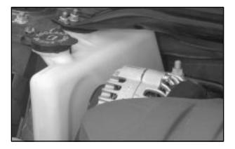
When the engine is cold, the coolant level should be at or above the COLD mark on the coolant recovery tank. To check the coolant level, look for the COLD mark on the side of the coolant recovery tank that faces the engine. Check to make sure that the coolant level is up to the COLD fill level on the side of the coolant recovery tank. If it isn't, you may have a leak in the radiator hoses, heater hoses, radiator, water pump or somewhere else in the cooling system.
