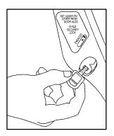
On the inside of the rear door will be a lock. Insert your key into this lock and turn it upward. This will engage the safety lock. To disengage the feature, turn the lock downward.
