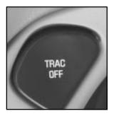
To turn the system on or off, press the TRAC OFF button on the left side of the instrument panel.
