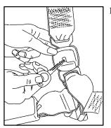
1. Remove the rear center lap-shoulder belt latch by using a key to press the release button.
