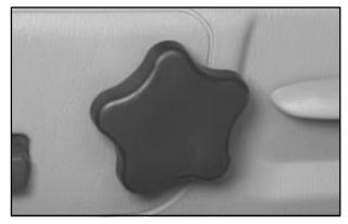
The knob that controls this feature is located on the outboard side of the driver's seat. Turn the knob toward the front of the vehicle to increase lumbar support. Turn the knob toward the rear of the vehicle to decrease lumbar support.
