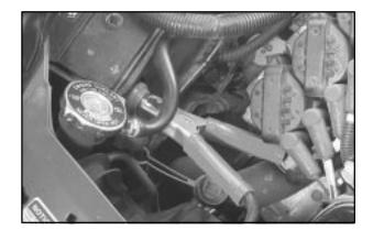
6. Connect the red positive (+) cable to the positive (+) terminal of the vehicle with the dead battery. Use a remote positive (+) terminal if the vehicle has one.
