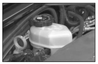
Your brake master cylinder reservoir is on the driver's side of the engine compartment. See "Engine Compartment Overview" in the Index. It is filled with DOT-3 brake fluid.
