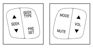
**SEEK:** Press the up arrow to tune to the next radio station and the down arrow to tune to the previous radio station.
