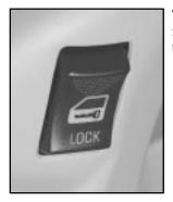
The power door lock switch is located on the door above the armrest.
