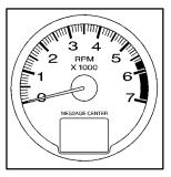
The tachometer displays the engine speed in thousands of revolutions per minute (rpm). (3800 V6 engine cluster tachometer shown.)
