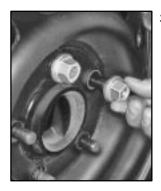
5. Reinstall the wheel nuts with the rounded end of the nuts toward the wheel. Tighten each nut by hand until the wheel is held against the hub.
