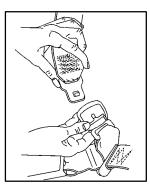
2. Reconnect the center safety belt latch plate to the buckle.
