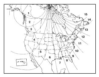
Turn the ignition on and cycle the DIC to the Compass/Temperature mode. Press the RESET button for approximately five seconds. The last entered variance zone number and "VAR" will be displayed. Press the MODE button until the proper variance number on the map is shown. Press the RESET button to set the new variance zone and resume normal operation.
