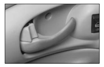
To lock the door from the inside, push the manual lock lever forward. To unlock, pull the lever rearward.
