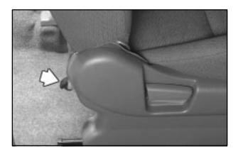
To get out, push the release pedal on the rear of the passenger's side front seat. Then tilt the seatback forward, and slide the whole seat forward.
