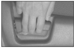
To adjust the seatback, lift the lever on the outboard side of the seat cushion. Release the lever to lock the seatback where you want it. Pull up on the lever, and the seat will go to its original upright position.
