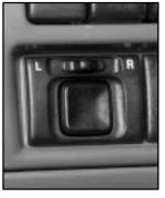
The switch to control the power mirrors is located on the lower left side of the instrument panel.
