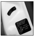
Your vehicle is equipped with rear door security locks that help prevent passengers from opening the rear doors of your vehicle from the inside. The rear security door locks are located on the inside of the rear doors.
