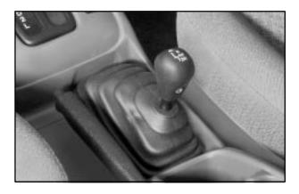
The transfer case shift lever is on the floor to the right of the driver. Use this lever to shift into and out of four-wheel drive. An indicator light comes on when the transfer case is in four-wheel drive. **TWO-WHEEL HIGH (2H):** This setting is for driving in most street and highway situations. Your front axle is not engaged in two-wheel drive.
