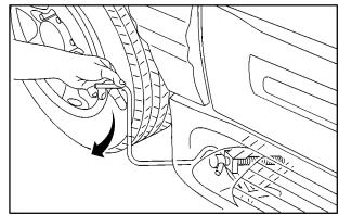
3. Raise the vehicle by turning the jack handle clockwise. Raise the vehicle far enough off the ground so there is enough room for the spare tire to fit underneath the wheel well.
