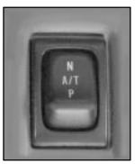
A power mode selector switch is included with the four-speed automatic transmission.
