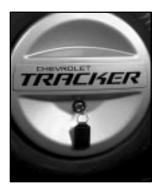
3. The spare tire is mounted on your tailgate. Your vehicle may be equipped with a cover. To remove the cover from the spare tire, insert your key into the wheel lock and pull the wheel lock off.
