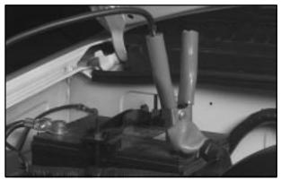
7. Don't let the other end touch metal. Connect it to the positive (+) terminal of the good battery. Use a remote positive (+) terminal if the vehicle has one.
