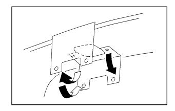
3. Unfasten the snaps that secure the canvas top to the roof. The snaps are located on either side of the dome lamp. Reattach the snaps which hold the sunroof canvas in place.
