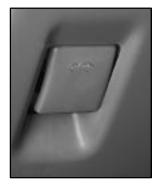
1. To open the hood, first pull the release handle located on the driver's side of the vehicle on the lower portion of the instrument panel.
