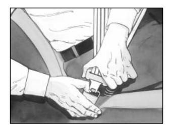
To unlatch the belt, just push the button on the buckle. The belt should go back out of the way.
