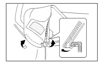
3. Loosen the lower rear corners of the convertible top.
