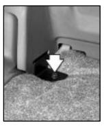
1. Remove the two attaching bolts from each lower corner of the cargo area.
