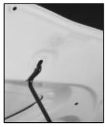
3. Lift the hood, release the hood prop from its retainer and put the hood prop into the slot in the hood.
