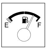
Your fuel gage shows about how much fuel is in your tank. When the gage first indicates "E" (empty), you still have about one or two gallons (4 to 8 L) of fuel left in your tank, but you need to get more right away.
