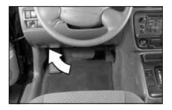
This fuse box is located under the driver's side of the instrument panel. The fuses here protect each separate circuit including headlamps. There are spare fuses inside the fuse box. If you have electrical failure, check here first.
