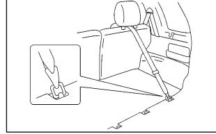
When routing the top strap at the center seating position, be sure to pass it between the rear seatbacks if the top strap connection to the child restraint is below the top of the rear seatback.
