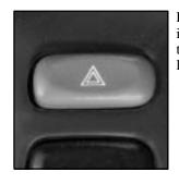
Press the button on the instrument panel to make the front and rear turn signal lamps flash on and off.
