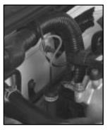
The automatic transmission dipstick has a red ring handle located in the rear of the engine compartment toward the center of the vehicle.
