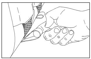
Pull the release straps located near the center of the vehicle to release the seat cushion. Fold the seat cushion forward.
