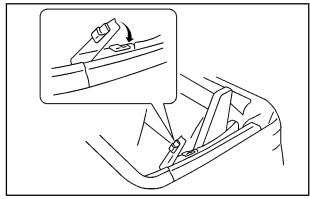
5. Engage the latches by pushing down on the support arms at the hinges.
