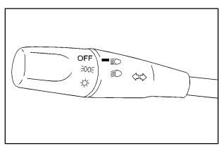
Turn the outside part of the lever to control the lamps. There are three positions for the lamp switch.
