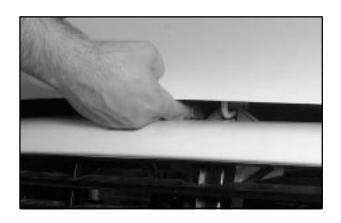
2. Then go to the front of the vehicle, pull up on the hood, and push the hood release lever to your right.
