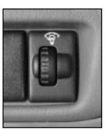
The thumbwheel controls the brightness of your instrument panel lights. Turn the wheel upward to brighten the lights or downward to dim them.
