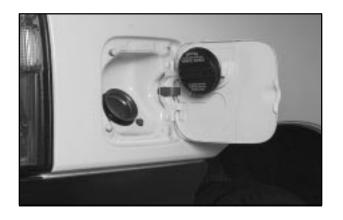
While refueling, place the cap in the holder provided. To remove the cap, turn it slowly to the left (counterclockwise).
