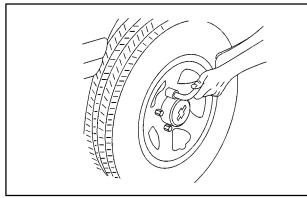
1. Using the wheel wrench, loosen all the wheel nuts, but don't remove them yet.
