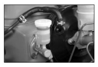
Refer to the Maintenance Schedule to determine how often you should check the fluid level in your clutch master cylinder reservoir and for the proper fluid. See "Owner Checks and Services" and "Recommended Fluids and Lubricants" in the Index.
