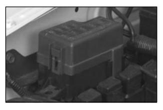
The main fuse box in your engine compartment protects all electrical loads. See "Engine Compartment Overview" in the Index for more information on location.
