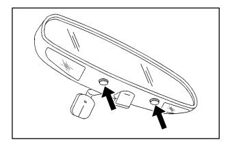
The mirror can also be adjusted for day or night driving. Pull the tab for night driving to reduce glare. Push the tab for daytime driving.
