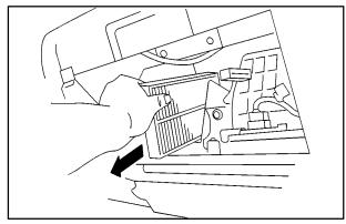
3. Remove the top air filter, then lift out the lower filter.
