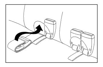
1. Fold the safety belt buckles and center safety belt (if equipped) into the pocket of the rear seatback.
