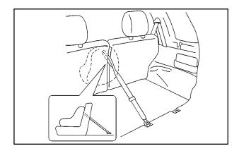
Anchor the top strap to one of these anchor points. Be sure to use an anchor point located on the same side of the vehicle as the seating position where the child restraint will be placed. Raise the head restraint and route the top strap under it.
