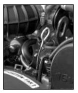
The handle of the engine oil dipstick is a round, yellow ring. On the 1.6L engine, it is located near the front of the engine compartment towards the passenger's side of the vehicle.
