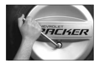
4. Using the wheel wrench, remove the wheel cover nut. Gently pry the spare tire cover off the wheel.
