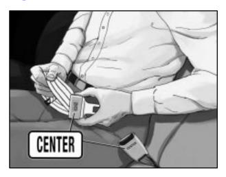
When you sit in the center seating position, you have a lap safety belt, which has no retractor. The word "CENTER" is on both the buckle and latch plate. Also, the center buckle and latch plate are a different color than the two outboard buckles and latch plates. To make the belt longer, tilt the latch plate and pull it along the belt.
