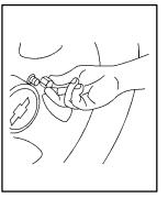
8. Reinstall the wheel nuts with the cone-shaped end of the nuts toward the wheel. Tighten each nut by hand until the wheel is held against the hub.
