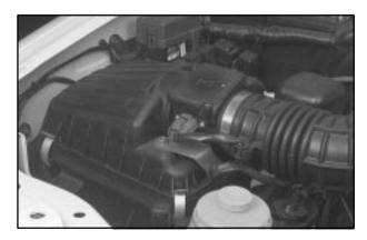
The engine air cleaner/filter is located on the passenger's side of the engine compartment toward the front of the vehicle. See "Engine Compartment Overview" in the Index for more information on location.
