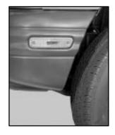
1. Remove the two screws holding the sidemarker lamp assembly using a screwdriver. The assembly should pull away from the vehicle.
