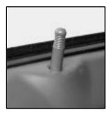
To lock the door from the inside, push down on the manual lock rod located on the door. To unlock it, pull up on the manual lock rod.
