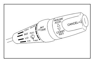
The lever on the right side of the steering column controls the windshield wipers and washers.
