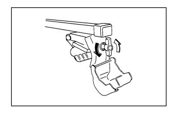
2. Turn the screw counterclockwise to loosen the mounting attachment so it can fit over the side rails.
