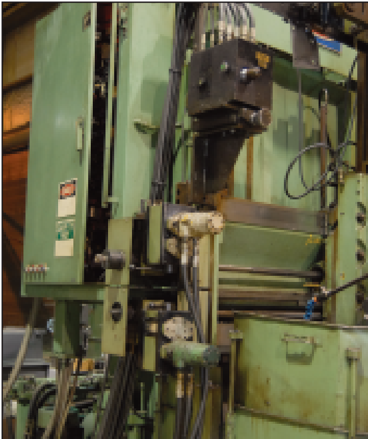
MIMIK HYDRAULIC TRACER ON DYNATROL ON BULLARD 36" VERTICAL TURRET LATHE
