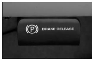
To release the parking brake, hold the regular brake pedal down. Pull the bottom edge of the lever, located above the parking brake pedal, marked BRAKE RELEASE, to release the parking brake.
