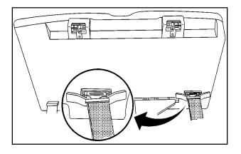
On all models with 60/40 split bench seats, you must insert the center occupant lap belt latch plate into the loop provided, on the underside of the folded forward seat cushion, before folding the rear seat back down on the driver's side.
