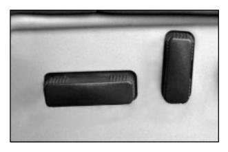
If your vehicle has a power seat, you can adjust it with these controls located on the outboard sides of the seats.
