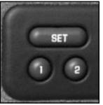
If your vehicle has this feature, the buttons used to program and recall the driver's seat and recliner position are located on the driver's door trim panel.
