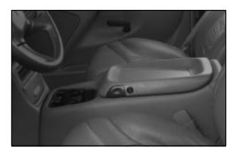
To open it, insert the console key into the lock and unlock the console. Press the button and swing the console lid open.
