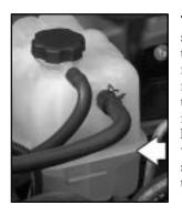
The coolant level should be at or above the FILL COLD mark. If it isn't, you may have a leak at the pressure cap or in the radiator hoses. heater hoses, radiator, water pump or somewhere else in the cooling system.
