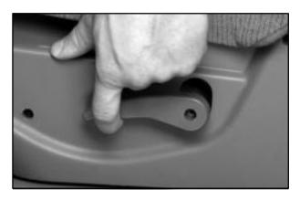
To adjust the front seatback, lift the manual lever located on the outboard side of the seat. Release the lever to lock the seatback where you want it. Lift the lever again without pushing on the seatback and the seatback will go to an upright position.
