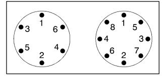
8. Tighten the nuts firmly in a crisscross sequence as shown by turning the wheel wrench clockwise.
