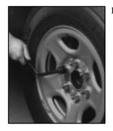
1. Use the wheel wrench to loosen all the wheel nuts. Turn the wheel wrench counterclockwise to loosen the wheel nuts. Don't remove the wheel nuts yet.
