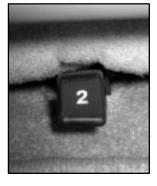
3. To unlatch the seat from the floor, pull up on the release lever labeled 2, located at the rear of the seat, and lift the rear of the seat up off the floor.
