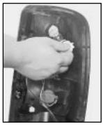
4. Pull the old bulb straight out from the socket.
