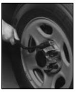
If your vehicle has wheel nut caps, loosen them by turning the wheel wrench counterclockwise. If you have a center cap with wheel nut caps, the wheel nut caps are designed to remain with the center cap. Remove the center cap.
