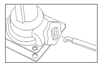
Attach the wheel wrench to the jack handle extensions (as needed). Attach the jack handle to the jack.
