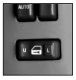
Press the raised side of the switch, marked L on either front door to lock all the doors at once.
