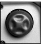
If your vehicle has this feature, the four-way control is located on the outboard side of the seat.
