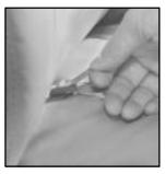
To fold, pull up on the strap loop at the rear of the seat cushion. Then, pull the seat cushion up an fold it forward.
