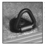
There are cargo tie downs in the rear cargo area that allow you to strap cargo in and keep it from moving inside the vehicle.
