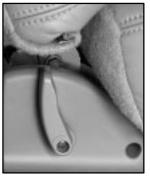
Push the seatback release lever rearward and pull the seatback forward. Then fold it until it is flat.
