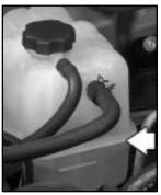
The coolant surge tank is located in the engine compartment on the passenger's side of the vehicle. See "Engine Compartment Overview" in the Index for more information on location.
