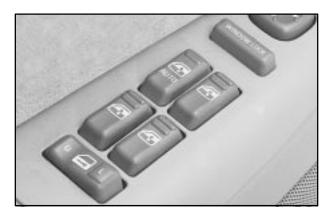
The driver's door has a switch for the passenger's windows as well. Your power windows will work when the ignition has been turned to ACCESSORY or RUN or when Retained Accessory Power (RAP) is active. See "Retained Accessory Power" in the Index.
