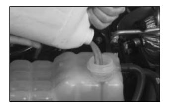
3. Then fill the coolant surge tank with the proper mixture, to the FILL COLD mark.
