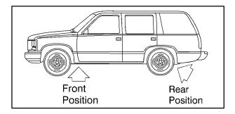
Position the jack under the vehicle. If the flat tire is on the front of the vehicle, position the jack on the frame behind the flat tire where the frame sections overlap.
