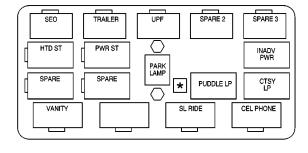
**Relay Name** Usage **SEO** Special Equipment Option HTD ST **Heated Seats SPARE** Not Used VANITY **Headliner Wiring** TRAILER Trailer Brake Wiring **PWR ST** Power Seats Not Used SPARE UPF Upfitter PARK LAMP Parking Lamps (Relay) FRT PRK EXPT\* Not Used SPARE 2 Not Used PUDDLE LP Puddle Lamps SL RIDE Not Used SPARE 3 Not Used **INADV PWR** Interior Lights Feed (Relay) CTSY LP Courtesy Lamps (Relay) **CEL PHONE** Cellular Telephone Wiring
