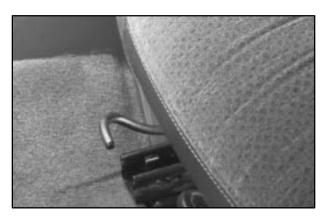
If your vehicle has this feature, you can raise or lower the front of the driver's or passenger's seat with this lever located at the inside edge of the seat. To raise or lower the front of the seat, move the lever up or down in a continuous motion until the cushion reaches the desired height.
