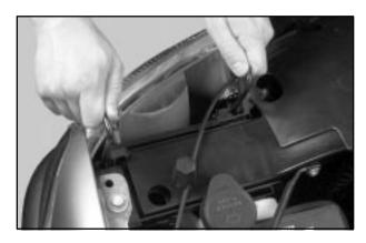
Remove the two pins on the top of the headlamp assembly. To remove the pins, turn the outer pin outward and pull it straight up. To remove the inner pin, turn it in and pull it straight up.
