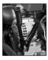
9. Connect the other end of the negative (-) cable to the negative (-) terminal of the dead battery or to a remote negative (-) terminal if the vehicle has one.
