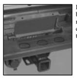
If you will be using the bumper to tow a trailer, you must remove the center cutout circle to install the trailer ball.
