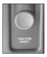
To turn the system on or off press the TAS on/off button located to the left of the steering wheel on the instrument panel.
