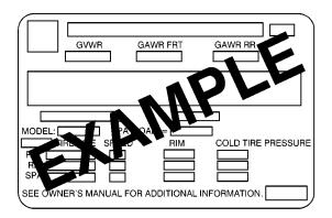
The Certification/Tire label is found on the rear edge of the driver's door or in the Incomplete Vehicle Document in the cab.
