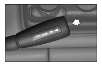
Your vehicle is equipped with a tow/haul mode. The selector button is located on the end of the column shift lever. You can use this feature to assist when towing or hauling a heavy load. See "Tow/Haul Mode" in the Index for more information.
