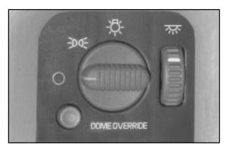
The control on the driver's side of your instrument panel operates the exterior lamps.
