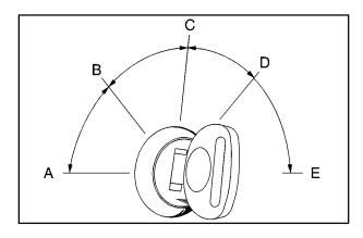
A (ACCESSORY): This position lets you use things like the radio, power windows and the windshield wipers when the engine is off. Push in the key and turn it toward you.
