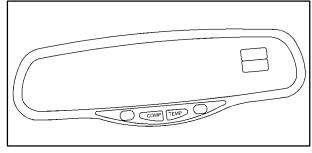
The mirror also includes a display of both the compass and the temperature in the upper right corner of the mirror face. The dual display can be turned on or off by briefly pressing either COMP or TEMP button.
