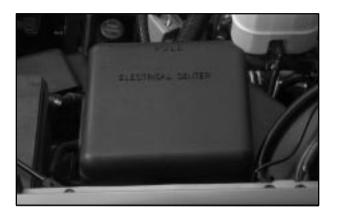
The underhood fuse block is located on the driver's side of the vehicle near the battery. Lift the cover for access to the fuse/relay block.
