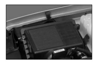
Your engine air cleaner/filter is located in the front corner of the engine compartment on the passenger's side of the vehicle. See "Engine Compartment Overview" in the Index for more information on location.
