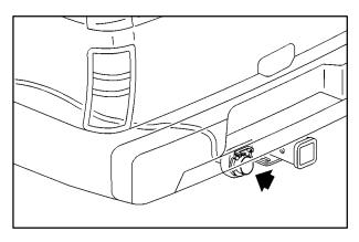
Your vehicle is equipped with the seven-wire trailer towing harness. This harness with a seven-pin universal heavy-duty trailer connector that is attached to a bracket on the hitch platform.
