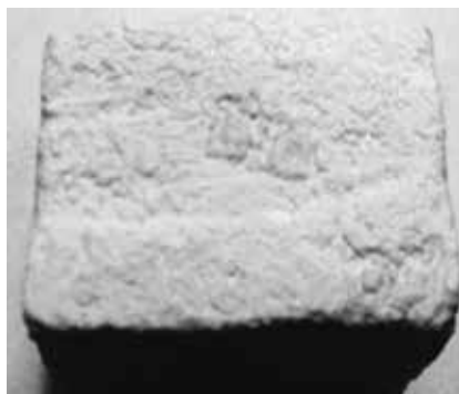
Figure 6 – A sample of the simulative core surface after modeling interaction of the retarded acid composition under formation conditions
