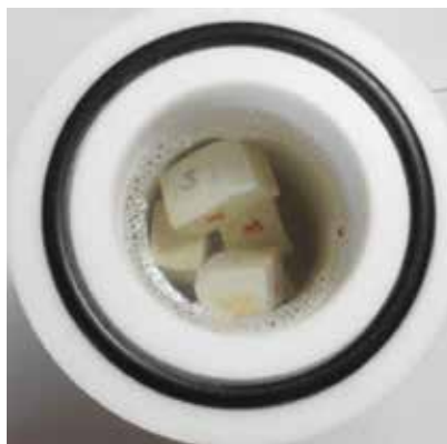
Figure 5 – Samples of the simulative core to determine the parameters of the kinetics of dissolution of the designed retarded acid composition in heat-proof and corrosion-resistant cell of high temperature thermochemical reactor
