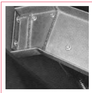
Stringer bolted solidly to top support.
