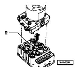
When pulling off control module, make sure that the hydraulic unit valve dome does not contact the control module solenoid valves.
