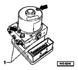
Remove E 5 hex socket head bolt -arrows- from hydraulic pump.
