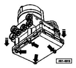
Remove bolts (arrows) from control module and remove control module.
