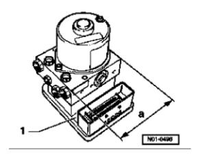
1. Control module, 47-pin (screwed to hydraulic unit). Two 4.8 mm wide contacts are located at both ends of the connection. The wiring linking between hydraulic unit and control module is routed internally.
