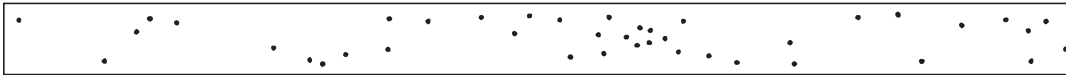
Typical Quantity and Size Permitted in 6 in. (150 mm) Length of Weld 1/8 in. (3 mm) to 1/4 in. (6 mm) Thickness
