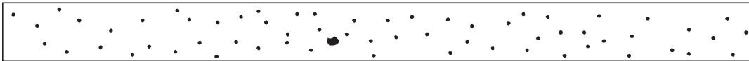
Typical Quantity and Size Permitted in 6 in. (150 mm) Length of Weld Over 1/4 in. (6 mm) to 1/2 in. (13 mm) Thickness
