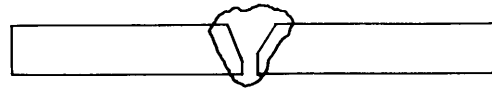
QW-463.2(b) PLATES — \frac{3}{4} in. (19 mm) AND OVER THICKNESS AND ALTERNATE FROM \frac{3}{8} in. (10 mm) BUT LESS THAN \frac{3}{4} in. (19 mm) THICKNESS PERFORMANCE QUALIFICATION
