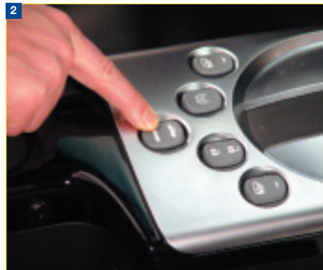
2 Press and hold the power top control button that is located on the center console.
