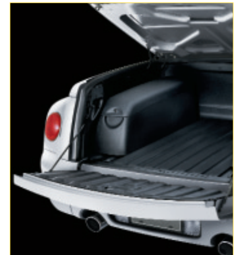
Integrated Side-Saddle Storage (RPA RAE) Includes two lockable storage boxes that are form-fitted and attach to the floor and side tracks.
