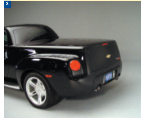
3 In the event of power loss, a manual release for the cargo cover is located underneath the vehicle behind the driver's-side rear wheel. See the Owner's Manual for instructions.
