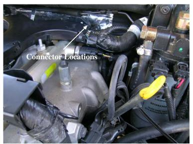
2. Disconnect the stock wiring harness connector at the MAP sensor. The MAP sensor is located on top of the of the intake manifold towards the rear of the engine on the driver's side. The intake manifold is located on top of the engine. It may be necessary to move the plastic race that holds the harness on top of the engine up in order to reach the Map sensor connector. Plug the supplied MAP sensor
