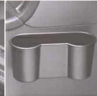
Waste/storage box – fitted on the passenger side of the centre tunnel. Designed as a holder for two soft-drink cans. Five CD discs can be stored in the middle section; can alternatively be used as a holder for a waste bag. ■ ◆ ▶ ▼ ▲ ● ○
