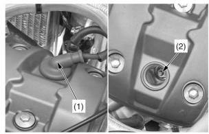
(1) spark plug cap(2) spark plug
