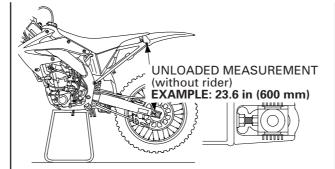
3. Measure the *loaded with rider* dimension. Remove the workstand. With two helpers available, sit as far forward as possible on your CRF's seat, wearing your riding apparel. Ask one helper to steady your CRF perfectly upright so you can put both feet on the pegs. Bounce your weight on the seat a couple of times to help the suspension overcome any situation and settle to a good reference point.
