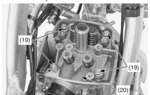
(19) cylinder head nuts/washers(20) cylinder head
