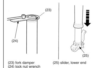
15. Pour the fork oil from the outer tube (20). Pour the fork oil from the oil hole (26) of the fork damper.
