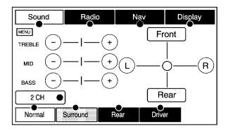
Press the MENU hard key to adjust several of your system's features and preferences. The last selected menu screen will be the screen that displays (Sound, Radio, Nav (navigation), or Display).
