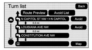
$\wedge$  / $\vee$  (Scroll Arrows): Touch the up and down arrow screen buttons to scroll through the list of maneuvers.
