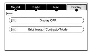
Press the MENU key to enter the Menu options, then press the MENU key to select Display or touch the Display screen button.
