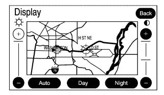
Touch this screen button to change the brightness, contrast, and mode of the display.
