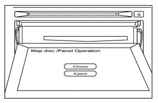
Once the map DVD is loaded and the Eject screen button is active, touch the Close screen button. The screen will close.
