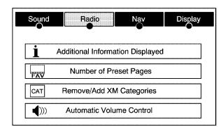
Press the MENU key to enter the menu screen, then press the MENU key repeatedly until Radio is selected or touch the Radio screen button to make changes for radio information displayed, number of preset pages, XM categories, and Automatic Volume Control or Bose<sup>®</sup> AudioPilot<sup>®</sup>.
