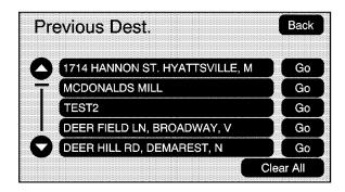
(Previous Destination): Touch this screen button to access the Previous Dest. screen. The system will store up to 100 points that have been previously input. As new destinations are entered, the system will automatically delete the oldest destinations and add the new destinations. To use the previous destination entry method, do the following:
