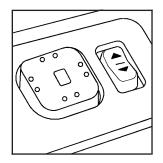
If your vehicle is equipped with power outside mirrors, the controls are located on the driver's door armrest.
