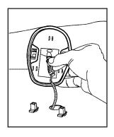
Install a new bulb into the socket and turn clockwise until it locks into place.
