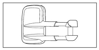
If your vehicle is equipped with this trailer towing type mirror, they can be adjusted so you can have a clear view of the objects behind you. Pull out the mirror head to extend it for better visibility when towing a trailer.
