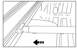
3. Remove the three bows by gently pushing them against the spring-loaded end. The three bows are labeled front, center, rear to remind you of the order in which to reinstall them.
