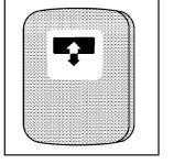
The sunroof control is located on the overhead console. Press the rear of the control to open the sunroof to the vent position, then press the rear of the control again to express-open the sunroof.
