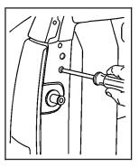
Remove the two rear lamp assembly screws near the tailgate latch and pull out the lamp assembly. 3. Determine which of the following taillamp assembly applies to your vehicle.
