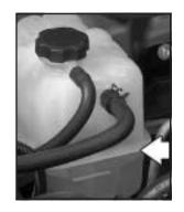
The coolant level should be at or above the FULL COLD mark. If it is not, you may have a leak at the pressure cap or in the radiator hoses, heater hoses, radiator, water pump, or somewhere else in the cooling system.
