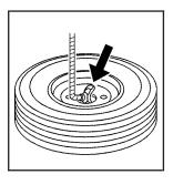
Tilt the retainer at the end of the cable when the tire has been lowered, so it can be pulled up through the wheel opening.
