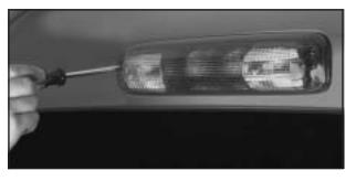
1. Remove the screws and lift off the lamp assembly.
