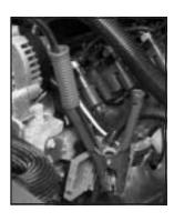
7. Connect the red positive (+) cable to the positive (+) terminal of the vehicle with the dead battery. Use a remote positive (+) terminal if the vehicle has one.
