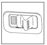
To lock the door from the inside, slide the lever rearward. To unlock the door, slide the lever forward
