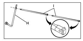
Attach the wheel wrench (H) and extensions (I) together.
