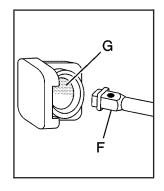
Insert the hoist end (open end) (F) of the extension through the hole (G) in the rear bumper.
