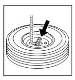
15. Tilt the retainer at the end of the cable and pull it through the wheel opening. Pull the tire out from under the vehicle.
