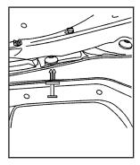
Pull the push-pins and lower dam assembly away from the retainers until the lower dam is free.
