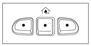
The Universal Home Remote System, a combined universal transmitter and receiver, provides a way to replace up to three hand-held transmitters used to activate devices such as gate operators, garage door openers, entry door locks, security systems, and home lighting.
