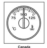
This gage shows the engine coolant temperature.
