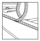
To remove, unsnap the cover. Roll it up and stow it using the buckle and the strap located at the front of the box.
