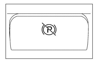
To release the parking brake, hold the regular brake pedal down. Pull the bottom edge of the lever, located above the parking brake pedal, with the parking brake symbol, to release the parking brake.
