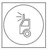
This button is located on the center of the instrument panel near the climate controls. When the wiring is connected to an auxiliary roof mounted lamp, pressing the button will activate the lamp and illuminate an indicator light near the button. Pressing the button again will turn off the roof mounted lamp.
