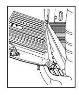
2. With the tailgate at a slight upward angle, pull back on the tailgate at the right edge and then move the tailgate to the right to release the left edge.
