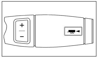
If your vehicle has an Allison Transmission®, it may have a Tow/Haul mode. Tow/Haul mode adjusts the transmission shift pattern to reduce shift cycling, providing increased performance, vehicle control, and transmission cooling when towing or hauling heavy loads.
