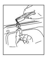
While continuing to pull downward on the push-pin, squeeze and turn the expandable end of the push-pin with a tool until it releases from the retainer.
