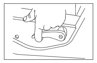
To adjust the seatback, lift the manual lever located on the outboard side of the seat. Release the lever to lock the seatback in the desired position. Lift the lever again without pushing on the seatback and the seatback will go to an upright position. If your vehicle has power seats with a power recliner, see *Power Seats on page 1-4* for further information on how to operate the reclining seatback feature.
