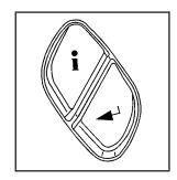
(Trip Information): Press this button to display the odometer, trip odometers, timer, engine hours, and selected range if your vehicle has an Allison Transmission®.
