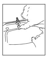
Push the flat end of the push-pin toward the retainer until it locks into place, making sure each is secure.
