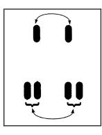
If your vehicle has dual rear wheels and the tread design for the front tires is different from the dual rear tires, always use the correct rotation pattern shown here when rotating your tires.
