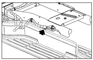
For vehicles not equipped with heavy duty trailering, the harness is clipped to the vehicle's frame behind the spare tire mount. The harness requires the installation of a trailer connector, which is available through your dealer.
