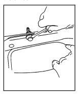
Insert a tool into the push-pin slot and pull downward until the push-pin snaps loose.
