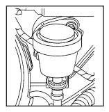
The clutch master cylinder reservoir is located in the rear of the engine compartment on the driver's side of the vehicle. See *Engine Compartment Overview on page 5-14* for more information on location.
