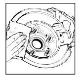
Remove any rust or dirt from the wheel bolts, mounting surfaces, and spare wheel. 8. Install the spare tire.
