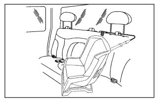
2.1. When using a child restraint with a top tether in the rear driver's side position, raise the head restraint and route the top tether through the fabric loop and under the center shoulder belt. Then, attach the top tether to the metal anchor point at the center rear seating position.
