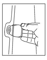
Your vehicle may have swing-out windows. To open a rear swing-out window, flip the latch open and swing the glass out.
