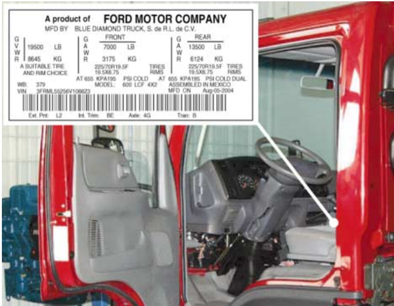
Vehicle Identification Label is located on the driver's side B-pillar
