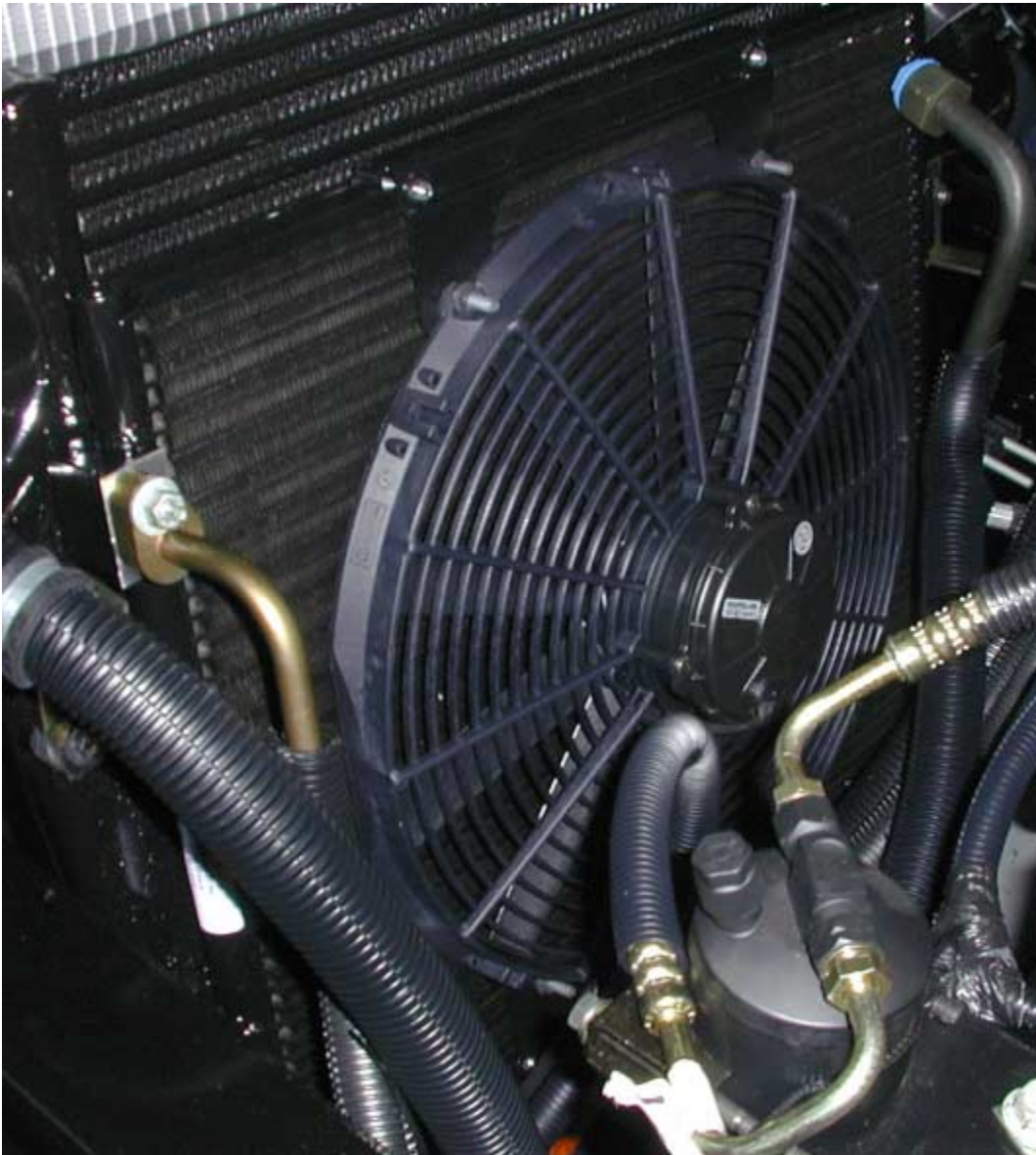
The LCF HVAC system is a typically system that also includes a pusher fan.
