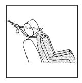
If the position you are using has a fixed headrest and you are using a dual tether, route the tether around the head restraint.
