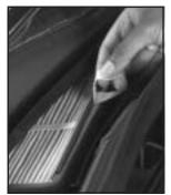
Remove the old air filter by pulling up on its tab.
