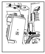
3.8L V6 Engine shown, 3.6L V6 Engine similar The coolant recovery tank is located in the engine compartment toward the rear of the engine on the passenger's side of the vehicle. See Engine Compartment Overview on page 350 for more information on location. The vehicle must be on a level surface when checking the coolant level.
