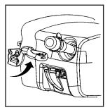
The lever that makes this adjustment is located on the left side of the steering column and behind the tilt lever, if the vehicle has this feature.
