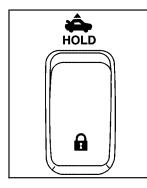
To lock or unlock all doors from inside the vehicle, use the power door lock switch located on either front door armrest.
