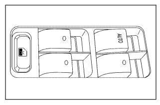
The switches on the driver's door armrest are used to control each of the windows. The power window switches work while the ignition is in RUN, ACCESSORY, or while Retained Accessory Power (RAP) is active. See *Retained Accessory Power (RAP) on page 110.* Each passenger door has its own window switch.
