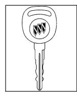
Your vehicle is equipped with PASS-Key<sup>®</sup> III (Personalized Automotive Security System) theft-deterrent system.
