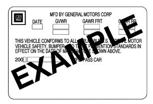
A vehicle specific Certification label is found on the rear edge of the driver's door. The label shows the gross weight capacity of your vehicle, called the Gross Vehicle Weight Rating (GVWR). The GVWR includes the weight of the vehicle, all occupants, fuel, and cargo.
