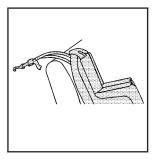
If the position you are using does not have a headrest and you are using a dual tether, route the tether over the seatback.
