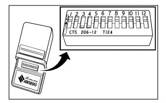
If you do not know if your garage door opener is a fixed code or rolling code device, open your garage door opener's remote control battery cover. Your garage door opener is a fixed code device if there is a panel of switches. If not, your garage door opener is a rolling code device.
