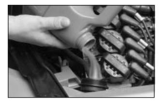
Fill the radiator with the proper DEX-COOL<sup>®</sup> coolant mixture, up to the base of the filler neck. See *Engine Coolant on page 363* for more information about the proper coolant mixture.
