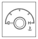
The vehicle has a gage that shows the engine coolant temperature.
