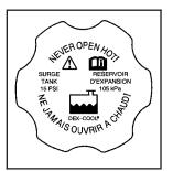
1. You can remove the radiator pressure cap when the cooling system, including the radiator pressure cap and upper radiator hose, is no longer hot.
