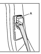
To move it down, press down on the release lever (A) and move the height adjuster to the desired position. You can move the height adjuster up just by pressing up on the shoulder belt guide.
