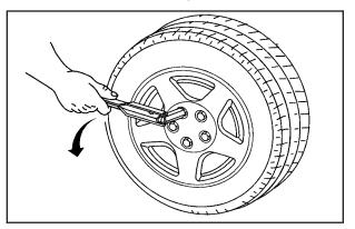
**Removing the Wheel Nuts**
