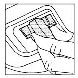
The lever that allows you to tilt the steering wheel is located on the left side of the steering column.
