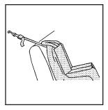
If the position you are using does not have a headrest and you are using a single tether, route the tether over the seatback.
