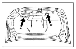
Your vehicle has a trunk lid pull down handle (A) located on the inside of the trunk lid on the driver's side of the vehicle. Use the handle to pull down the trunk lid when closing it.
