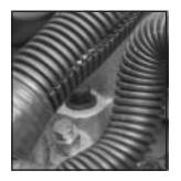
Open the coolant air bleed valve located on the thermostat housing, near the upper radiator hose.
