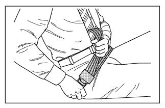
To make the belt shorter, pull its free end as shown until the belt is snug.
