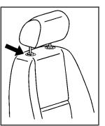
Pull the head restraint up to raise it. To lower the head restraint, press the release button, located on the top of the seatback, while you push the head restraint down.
