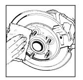
7. Remove any rust or dirt from the wheel bolts, mounting surfaces, and spare wheel.
