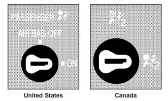
If your vehicle does not have an airbag off switch, it may have a passenger sensing system. See *Passenger Sensing System on page 103*. This switch should only be turned to the off position if the person in the right front passenger's position is a member of a passenger risk group identified by the national government as follows:
