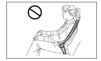
Wherever the child sits, the lap portion of the belt should be worn low and snug on the hips, just touching the child's thighs. This applies belt force to the child's pelvic bones in a crash.
