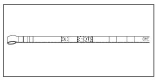
5. If the fluid level is below the COLD check band, add only enough fluid as necessary to bring the level into the COLD band. It does not take much fluid, generally less than one pint (0.5L). Do not overfill.
