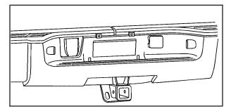
For vehicles equipped with heavy duty trailering, the harness is connected to a bracket on the hitch platform. The seven-wire harness contains the following trailer circuits:
