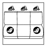
Crew and Extended Cab Rear Seat (Top Tether Anchor): Seating positions with top tether anchors.
