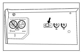
2. Locate in the garage, the garage door opener receiver (motor-head unit). Locate the "Learn" or "Smart" button. It can usually be found where the hanging antenna wire is attached to the motor-head unit and may be a colored button. Press this button. After you press this button, you will have 30 seconds to complete the following steps.
