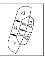
If your vehicle has audio steering wheel controls, they could differ depending on the vehicle's options. Some audio controls can be adjusted at the steering wheel. They include the following:
