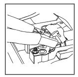
Connect the red positive (+) cable to the positive (+) terminal of the vehicle with the dead battery.
