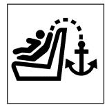
For regular cab models, there is an anchor symbol on the trim covers to assist you in locating the top tether anchors.
