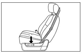
If the seats have power reclining seatbacks, the control used to recline them is located on the outboard side of the seat behind the power seat control.
