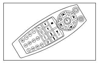
$\bigcirc$  (**Power**): Press this button to turn the video screen on and off.
