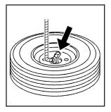
2. Tilt the retainer downward and through the wheel opening. Make sure the retainer is fully seated across the underside of the wheel.
