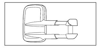
If your vehicle has trailer towing type mirrors, they can be adjusted so you can have a clear view of the objects behind you. Manually pull out the mirror head to extend it for better visibility when towing a trailer. These mirrors can be manually folded forward or rearward. The lower portion of the mirror is convex. A convex mirror's surface is curved so you can see more from the driver's seat. The convex mirror can be adjusted manually to the driver's preferred position for better vision.
