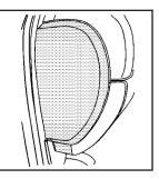
The instrument panel fuse block access door is located on the driver's side edge of the instrument panel.
