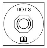
The brake master cylinder reservoir is filled with DOT-3 brake fluid. See *Engine Compartment Overview on page 506* for the location of the reservoir.
