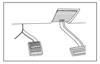
To release the parking brake, hold the regular brake pedal down. Then pull the bottom edge of the lever, with the parking brake symbol and located above the parking brake pedal. If the ignition is on when the parking brake is released, the brake system warning light goes off.
