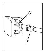
Insert the hoist end (F) through the hole (G) in the rear bumper and onto the hoist shaft (E).
