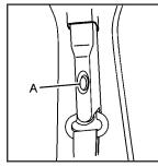
On the extended cabs, push down on the release button (A) and move the height adjuster to the desired position.
