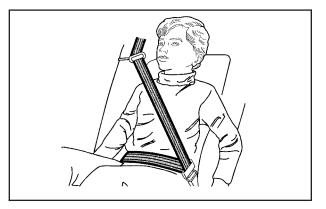
4. Buckle, position, and release the safety belt as described in *Rear Seat Passengers on page 39.* Make sure that the shoulder belt crosses the shoulder.
