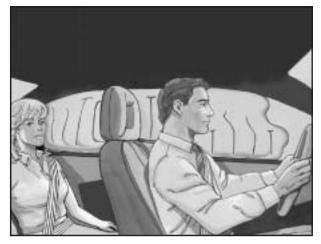
If your vehicle has a roof-mounted rollover airbag for the driver and the person seated directly behind the driver, it is located in the ceiling above the side windows.
