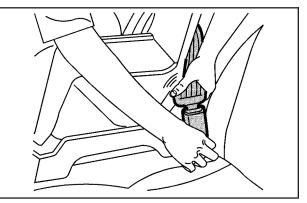
Buckle the belt. Make sure the release button is positioned so you would be able to unbuckle the safety belt quickly if you ever had to.
