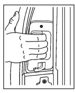
To open a rear access door from the outside, first open the front door. Then, use the handle located on the front edge of the rear access door to open it.
