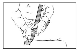
To unlatch the belt, push the button on the buckle.
