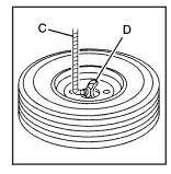
5. Use the wheel wrench hook which allows you to pull the hoist cable towards you to assist in reaching the spare tire.
