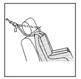
If the position you are using has an adjustable head restraint and you are using a dual tether, route the tether around the head restraint.
