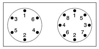
12. Tighten the nuts firmly in a crisscross sequence as shown by turning the wheel wrench clockwise.
