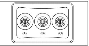
The A/V jacks, located on the rear of the floor console, allow audio or video signals to be connected from an auxiliary device such as a camcorder or a video game unit to the RSE system. Adapter connectors or cables could be required to connect the auxiliary device to the A/V jacks. Refer to the manufacturer's instructions for proper usage.
