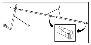
Assemble the wheel wrench (H) and the two jack handle extensions (I) as shown.
