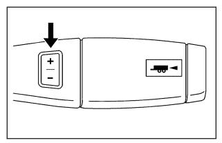
Your vehicle may have a Range Selection Mode. The Range Selection Mode helps control the vehicle's transmission and vehicle speed while driving down hill or towing a trailer by letting you select a desired range of gears. To use this feature, do the following:
