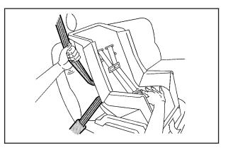
6. To tighten the belt, push down on the child restraint, pull the shoulder belt to tighten the lap belt portion, and feed the shoulder belt back into the retractor. If you are using a forward-facing child restraint, you may find it helpful to use your knee to push down on the child restraint as you tighten the belt. You should not be able to pull more of the belt out of the retractor once the lock has been set.
