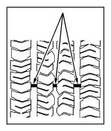
One way to tell when it is time for new tires is to check the treadwear indicators, which appear when your tires have only 1/16 inch (1.6 mm) or less of tread remaining. Some commercial truck tires may not have treadwear indicators. You need a new tire if any of the following statements are true:
