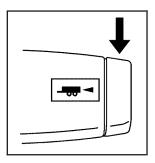
Press this button at the end of the shift lever to enable/disable the tow/haul mode.
