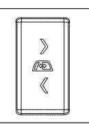
On vehicles equipped with a power sliding rear window, the switch is located in the overhead console. The power sliding rear window will work when the ignition has been turned to ACCESSORY, RUN, or when Retained Accessory Power (RAP) is active. See *Retained Accessory Power* (*RAP*) on page 141 for more information.
