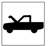
1. Pull the handle with this symbol on it. It is located inside the vehicle to the left of the brake pedal.
