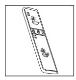
On vehicles with heated front seats, the controls are located on the driver's and passenger's doors, near the door handle. \* (Heated Seatback): Press this button to turn on the heated seatback.
