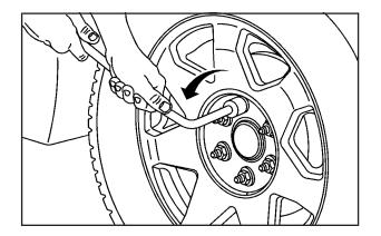
3. Use the wheel wrench and turn it counterclockwise to loosen the wheel nuts. Do not remove the wheel nuts yet.
