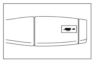
If your vehicle has an automatic transmission, it has a tow/haul mode. If your vehicle has an Allison or Hydra-Matic<sup>®</sup> 6-speed automatic transmission see "Tow/Haul Mode (Allison or Hydra-Matic<sup>®</sup> 6-Speed Automatic Transmission<sup>®</sup>) following. The tow/haul mode adjusts the transmission shift pattern to reduce shift cycling, providing increased performance, vehicle control, and transmission cooling when towing or hauling heavy loads.
