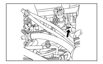
The remote negative (–) terminal is a stud located on the right front passenger side of the engine, where the negative battery cable attaches.
