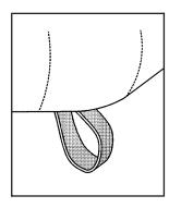
1. Pull up on the front of the seat cushion while pulling down on the release strap, located under the seat cushion.
