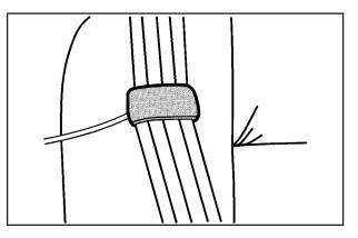
3. Be sure that the belt is not twisted and it lies flat. The elastic cord must be under the belt and the guide on top.
