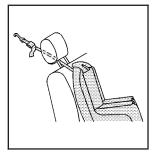
If the position you are using has an adjustable head restraint and you are using a single tether, raise the head restraint and route the tether under the head restraint and in between the head restraint posts.
