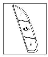
The controls for this feature are located on the driver's door panel, and are used to program and recall memory settings for the driver's seat, outside mirrors, and the adjustable throttle and brake pedal.
