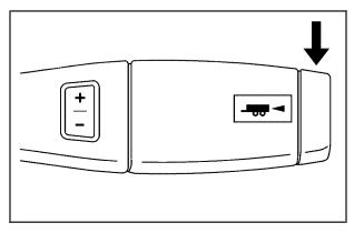
If your vehicle has an Allison or Hydra-Matic<sup>®</sup> 6-speed automatic transmission<sup>®</sup>, it has a tow/haul mode. The tow/haul mode adjusts the transmission shift pattern to reduce shift cycling, providing increased performance, vehicle control, and transmission cooling when towing or hauling heavy loads. Turn the tow/haul mode on and off by pressing the button, located on the end of the shift lever. When the tow/haul is on, a light on the instrument panel cluster will come on.
