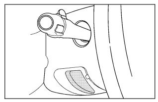
The tilt steering wheel lever is located on the lower left side of the steering column.
