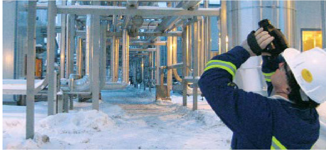
An operator uses the infrared camera to detect gas leaks too small to be seen by the human eye or sensed by traditional gas detection instrumentation. Piloted by the company in 2007, this technology will allow us to better maintain regulatory and environmental compliance, support our corporate responsibility emissions reporting, and increase operational efficiency.
