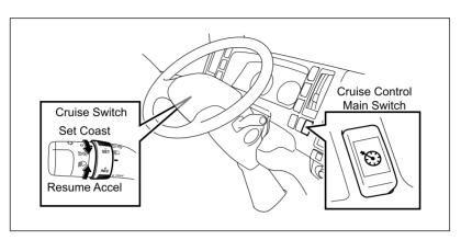
With cruise control, you can maintain a speed of between 30 and 75MPH (48 to 121 km/h) without keeping your foot on the accelerator pedal. At speeds below 30 MPH (48 km/h), the cruise control does not operate.
