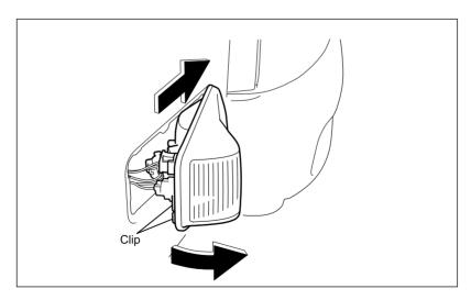
3. Upon removing the tabs, dismount the light by displacing it towards the back of the vehicle and pulling it out.
