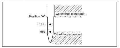
CAUTION: If the engine oil level is above the "FULL" mark of the dipstick, it may cause engine damage. Replace the engine oil if the oil level exceeds the "FULL" mark.
