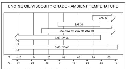
This Engine Oil Viscosity Grade Chart shows general information. For this vehicle, oil with \*W-40 viscosity is recommended.
