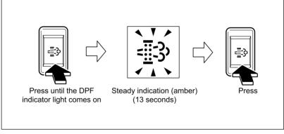
Confirm that the DPF indicator light (amber) is on for 3 seconds or longer, then press the DPF switch again while the DPF indicator light (amber) is on. NOTICE: Until a certain quantity of PM has accumulated in the DPF filter, the DPF indicator light (amber) will go off after 3 seconds, even if you continue to press the DPF switch. In this case, there is no need to perform DPF regeneration, so regeneration will not start even if you press the DPF switch.
