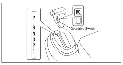
The overdrive will not operate when the overdrive switch is in the "OFF" position.
