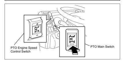
CAUTION: In PTO mode, Cruise Set/Resume Switch can be used exactly the same as PTO Engine Speed Control Switch. Improper operation of these switches may cause personal injury or damage.
