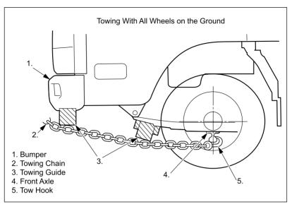
To prepare a disabled vehicle for front end towing with all wheels on the ground, the following steps are necessary:
