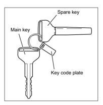
One key can operate all the locks on the vehicle. Keep one of the two keys provided as a spare. The key code is stamped on the tag.
