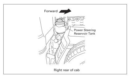
NOTICE: When replenishing power steering fluid or flushing the power steering system, always use ATF Fluid (DEXRON® -III). Failure to use the proper fluid may damage the power steering system seals and hoses, leading to fluid leakage.
