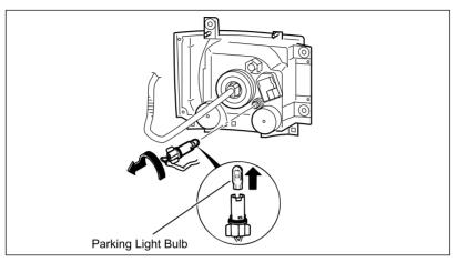
3. When installing, proceed in the reverse order while paying attention to the following points. Turn the connector to the right and lock securely.
