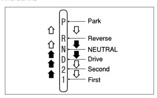
Push the button located on the end of the selector when engaging the "R" and "P" positions and when shifting from "2" to "1" as indicated by the arrow " ightharpoonup".
