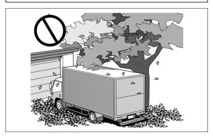
The Diesel Particulate Filter (DPF) is the system which purifies Particulate Matter (PM) in the exhaust gas. This collects PM into the DPF and regenerates the filter (burns PM) automatically.
