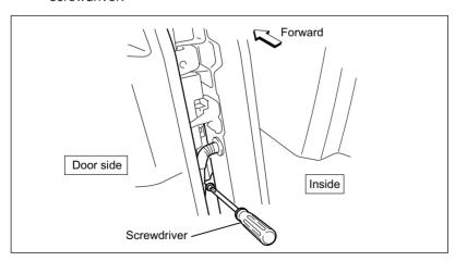
• Dismantle the entire turn signal light towards the front of the vehicle in an obliquely downward direction.
