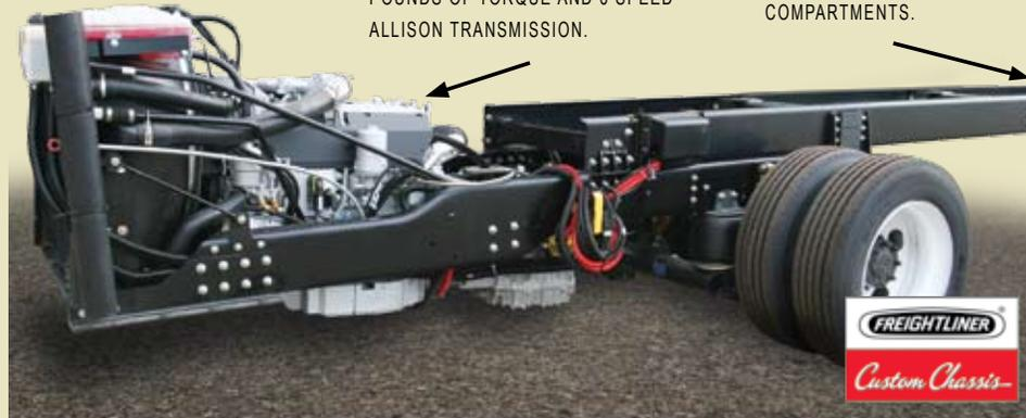
RAISED RAIL CHASSIS DESIGN ALLOWS FOR 7.5 FOOT INTERIOR CEILINGS AND MAXIMIZED BASEMENT STORAGE COMPARTMENTS.
