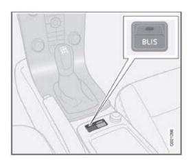
BLIS is automatically activated when the ignition is switched on. The indicator lights will provide confirmation by flashing 3 times.
