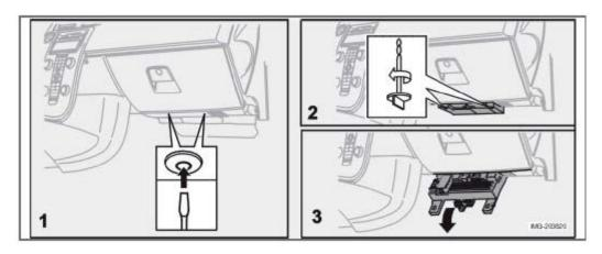
The fuse box in the passenger compartment is located under the glove compartment.
