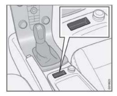
If the buttons for optional equipment are not installed, the recess behind the gear lever can be used as a storage compartment.
