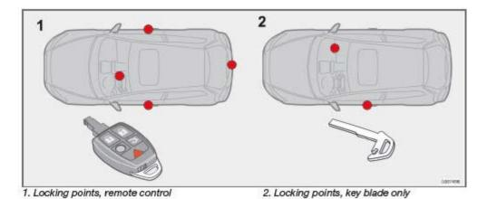
The key blade can be used to lock or unlock the vehicle or glove compartment (see page 127).
