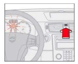
The four-way flasher should be used to indicate that the vehicle has become a traffic hazard. To activate the flashers, press the triangular button in the center dash. Press the button again to turn off the flashers.
