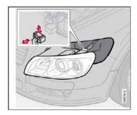
5. Disconnect the wiring connector by pressing and holding down the clip (3) with your thumb and pulling out the connector (4) with the other hand.
