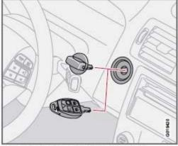
Removing the keyless drive start control
