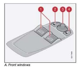
The power windows are opened and closed using the buttons in the armrests.
