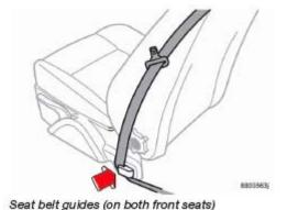
These guides are designed to help provide easier access to the seat belts. A belt can be taken out of the guide and slid to the rearmost part of the lower seat belt anchorage rod to make it easier for passengers to enter or exit the rear seat.
