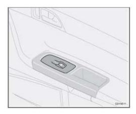
The control on the passenger's door open that window only.
