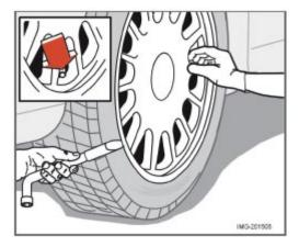
The spare tire, jack, and crank are located under the carpet on the floor of the cargo area.
