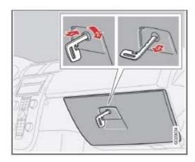
The glove compartment can only be locked and unlocked using the detachable key blade on the remote control. See page 119 for information on removing the key blade from the remote control.
