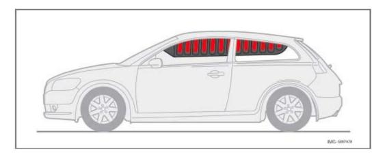
This system consists of inflatable curtains located along the sides of the roof liners, stretching from the center of both front side windows to the rear edge of the rear side windows. It is designed to help protect the heads of the occupants of the front and rear seats in certain side impact collisions.
