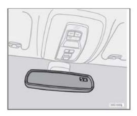
The upper right-hand corner of the rearview mirror has an integrated display that shows the compass direction toward which the vehicle is pointing. Eight different directions can be displayed: N, NE, E, SE, S, SW, W and NW. The display shows your car's orientation with respect to true north.
