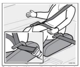
Position the child correctly on the booster cushion and fasten the seat belt
