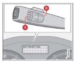
Controls on the left-side steering wheel lever
