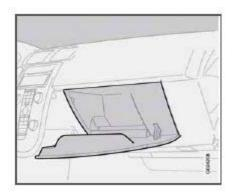
The owners manual and maps can be stored here. There are also holders for coins, pens and fuel cards. The glove compartment can only be locked and unlocked using the detachable key blade from the central locking system's remote control. See <u>page 120</u> for information on removing the key blade from the remote control, and <u>page 127</u> for information on locking the glove compartment.
