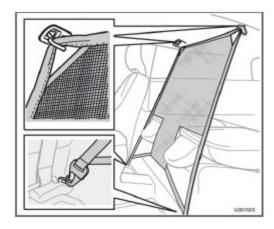
The cargo area net can be placed behind the front seat backrests. This net is only intended to be used when the rear seat backrests are folded down.
