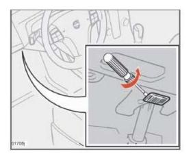
The footwell lighting is located under the dashboard on the driver's and passenger's sides. To replace a bulb:
