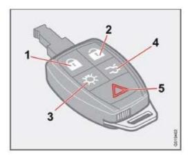
1. **Lock** - Press the Lock button on the remote once to lock all doors and the rear liftgate. The turn signals will flash once to confirm locking.
