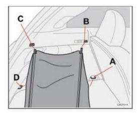
The cargo area cover is pulled over the cargo area and fastened to the eyelets with the hooks on the corners of the cover.
