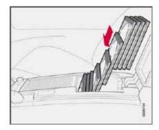
The deep storage compartment has room for 10 CD jewel cases. These cases must be inserted with their spines upward in order to allow space for 10 cases in the storage compartment.
