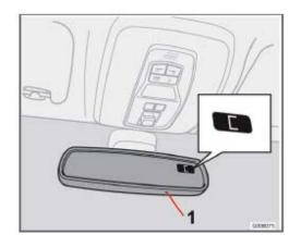
The compass may need to be calibrated in certain cases. If calibration is required, the character C appears in the mirror's display.
