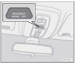
Occupant Weight Sensor (OWS) indicator light
