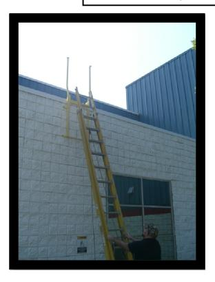
**LadderPort™**, the inexpensive permanent building mounted extension ladder receiver, securely holds the ladder in place. Hooks secure the ladder while side plates prevent it from moving left or right. The solid metal grab bars enable the technician to climb up and down a portable extension ladder comfortably and safely.
