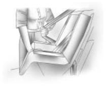
5. Pull the rest of the shoulder belt all the way out of the retractor to set the lock.
