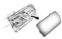
The rear compartment fuse block is located on the left side of the trunk behind a cover.
