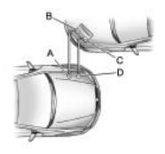
5. Connect one end of the red positive (+) cable to the jump start positive (+) post (A).
