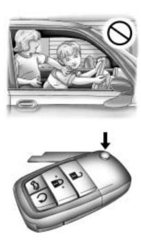
One key, located inside the Remote Keyless Entry (RKE) transmitter, can be used for the ignition and all locks except the glovebox.
