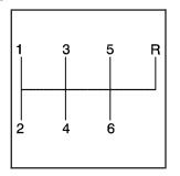
This is the shift pattern for the six-speed manual transmission.
