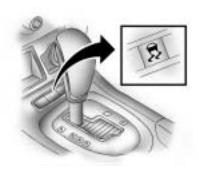
The ESP button is located in front of the transmission gear selector lever.
