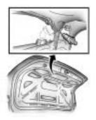
Turn the bulb socket counterclockwise and pull it straight out.
