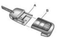
The key is purchased as two sections: the key blade and immobilizer section (A) and the remote keyless entry and remote start system section (B).
