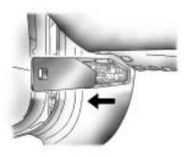
The instrument panel fuse block is located on the end of the instrument panel, on the driver side of the vehicle. To access the fuses, open the fuse panel door by pulling out.
