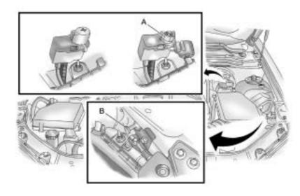
The jump start positive (A) and negative posts (B) are located in the engine compartment on the driver side of the vehicle. These posts are used instead of a direct connection to the battery.
