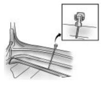
2. Pull the handle of the spare wheel cover strap straight up and secure to the trunk lid.
