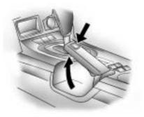
To set the parking brake, pull up on the parking brake handle. If the ignition is in the ON/RUN position, the brake system warning light will come on. See *Brake System Warning Light on page 4-15*.
