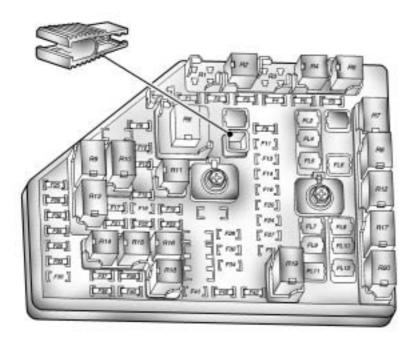
**Engine Compartment Fuse Block - Fuse Puller Shown**
