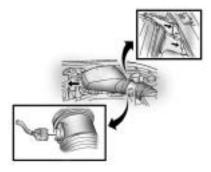
4. For the driver side remove the clip from the air cleaner/filter cover. Move the cover to the back, out of the way.
