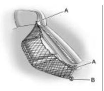
To create a pouch, attach the four corner loops (A) to each of the two top hooks. Attach the nets center loops (B) to the bottom hooks.
