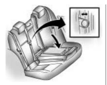
There is an emergency trunk release handle located inside the trunk on the trunk latch. Access the release handle by folding the rear seat center seatback. See *Rear Seat Operation on page 1-5.* Pull the release handle to open the trunk from the inside.
