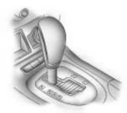
There are several different positions for the shift lever. When the position of the shift lever is changed, a message is shown in the Driver Information Center (DIC). The selected gear is magnified in the DIC, and changes according to the shift lever's movement. There are also messages for Sport Shift Mode, Normal Shift Mode and Driver Shift Control.
