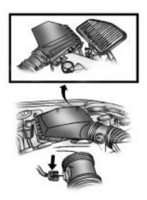
3. On the V8 engine, remove the airflow sensor connector by pushing in the tab and pulling straight back.
