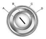
The ignition switch has four different positions.
