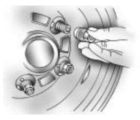
9. Remove all of the wheel nuts and place them in a dry, clean place to avoid getting dirt in the threads.
