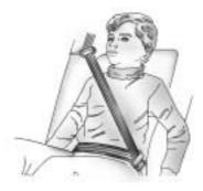
Buckle, position, and release the safety belt as described previously in this section. Make sure that the shoulder belt crosses the shoulder. To remove and store the comfort guide, squeeze the belt edges together so that the safety belt can be removed from the guide. Push the guide into the pocket on the side of the seatback.
