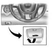
1. Pull the release handle with the above symbol on it. It is located below the instrument panel to the left of the steering wheel.
