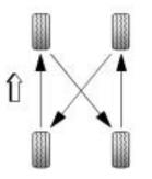
When rotating the vehicle's tires, always use the correct rotation pattern shown here.
