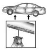
Position the jack lift head at the jack location nearest the flat tire. The location is indicated by a mark on the bottom edge of the vehicle. The jack must not be used in any other positions.
