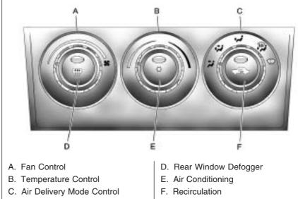
**(Fan Control):** Turn clockwise or counterclockwise to increase or decrease the fan speed. Turn the knob all the way counterclockwise to turn the system off.
