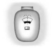
Open the cap with the washer symbol on it. Add washer fluid until the tank is full. See *Engine Compartment Overview on page 9-6* for reservoir location. Notice:
